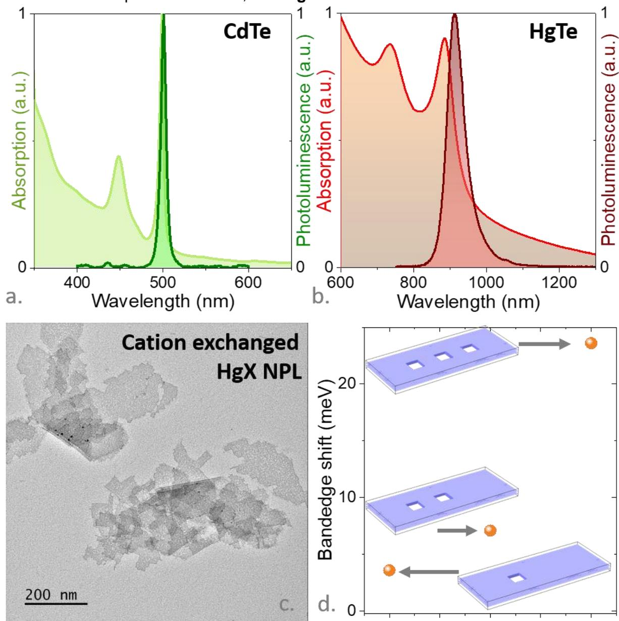
**Figure 1: HgTe NPL growth using cation exchange.** a. Absorption and PL spectra of 3 ML CdTe NPLs. b. Absorption and PL spectra of 3 ML HgTe NPLs. c. TEM image of 3 ML HgX NPLs using the procedure from ref 18 (X: Se or Te or a mix). d. Calculated shift of the band gap in the presence of geometric defects.
