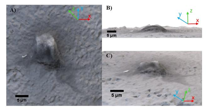
**Figure 1.** Top view (A), side view (B) and oblique view (C) of a reconstructed embryonic mouse fibroblast cell volume cultivated onto titanium from secondary electron images collected at different tilt angles.
