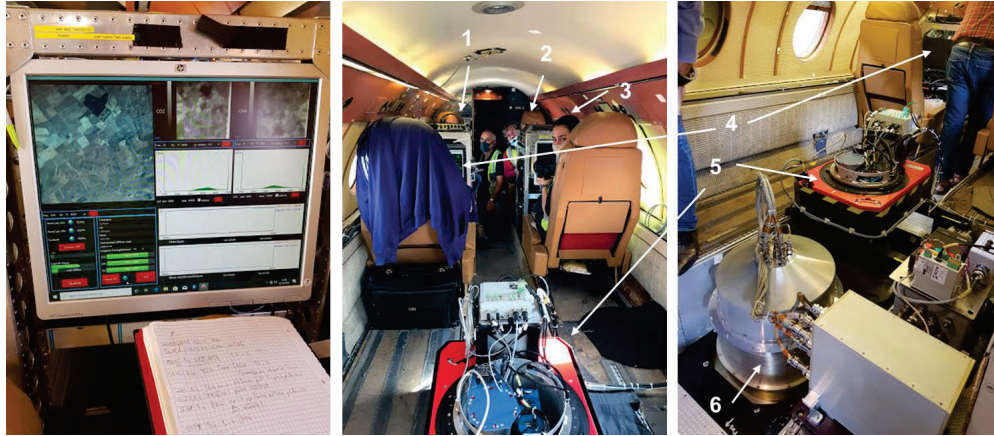
Figure 3. Left: NanoCarb user interface, seen from the NanoCarb operator seat. The image on the left is the visible image, while the two black and white images on the right are one thumbnail from the CO 2 and the CH 4 cameras. Middle and right: inside of the F20 1: Safire operator, 2: NanoCarb operator, 3: NanoCarb observer, 4: Spex operator, 5: GSM with the NanoCarb cameras, 6: SpexAirborne.
