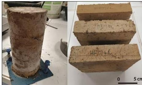
Fig. 7: Cylindrical and prismatic specimens
