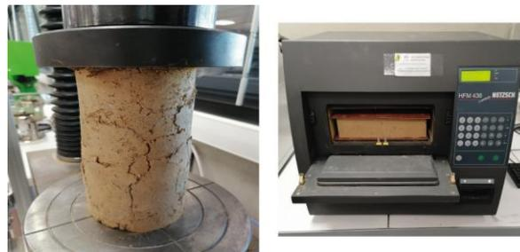
Fig. 8: Compressive strength test (Left) and thermal conductivity test (Right)
