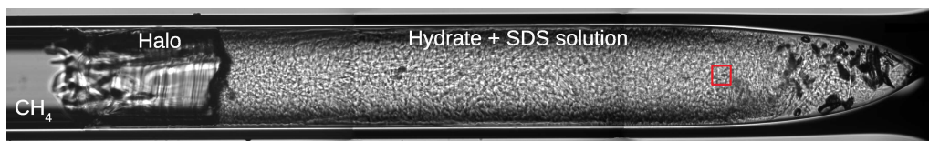
Figure 3: Transmission microscopy image of a porous methane hydrate in a glass capillary of diameter 200\ \mu\text{m} . The conversion lasted about 1 hour, starting on the meniscus and propagating to the capillary end on the right. Hydrate methane growth as a halo over the glass capillary wall is apparent near the meniscus. The red square is the region investigated by microRaman spectroscopy, see Figure 4.
