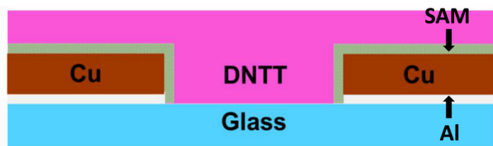
Fig. 2: Schematic and simplified diagram of diode formed by DNTT.
