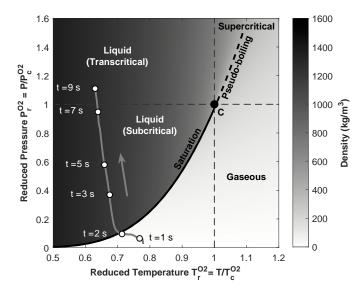
Figure 3: Trajectory (gray line) of the **Transcritical Case** in the Pressure-Temperature diagram of oxygen. The oxygen density is determined assuming a Peng-Robinson Equation of State.
