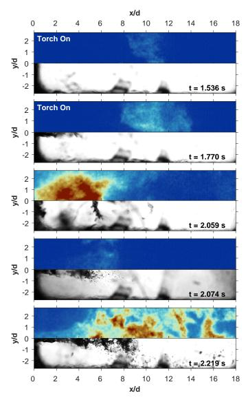
Figure 9: Series of **OH\* chemiluminescence** (top) and **backlit** (bottom) composite images of the **Subcritical** Case dynamically showing the oxygen-jet condensation and the flame anchoring at the central injector lip.
