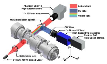
Figure 2: Schematic view of the dual high-speed visualization setup.
