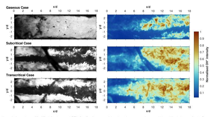
Figure 6: Comparisons of **backlit** (left column) and **OH\* chemiluminescence** (right column) instantaneous images (within stabilized plateaux) for the **Gaseous** (top row), **Subcritical** (middle row) and **Transcritical** (bottom row) cases.
