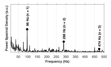
Figure 18: Fast Fourier Transform (FFT) of the oxygen feed line dynamic pressure recorded during the **Gaseous** Case stabilized plateau.
