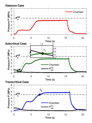
Figure 5: Evolution of the pressure in the combustion chamber for the **Gaseous** (top), **Subcritical** (middle) and **Transcritical** (bottom) cases.  $P_c^{O2}$ : oxygen critical pressure.  $P_s^{O2}$ : oxygen saturation pressure.
