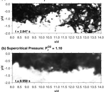
Figure 11: Closed-up views of the liquid-oxygen interface at **subcritical** (a) and **supercritical** (b) pressure.
