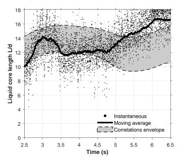
Figure 22: Evolution of the liquid core length L (**Subcritical** Case) compared to that evaluated based on the semi-empirical correlations of Mayer [62], Eroglu et al. [79] and Davis and Chehroudi [80].
