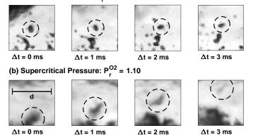
Figure 12: Single-droplet evolution at **subcritical (a)** and **supercritical (b)** pressure. Tracking of the droplets is performed on the 15-kHz-recording of the Transcritical Case 2. The frame of reference is moving with the droplet.  $\Delta t$ : local time frame. *d* is the injector inner tube diameter.
