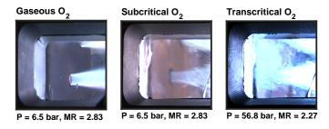
Figure 4: True-colors visualizations of the combustor for conditions of **gaseous** (left), **subcritical** (middle) and **transcritical** (right) oxygen injection.
