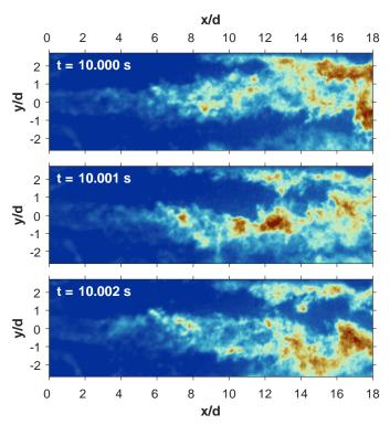
Figure 16: Series of OH\* chemiluminescence snapshots recorded during the stabilized plateau of the **Gaseous** Case. The time interval between snapshots is 1 ms.
