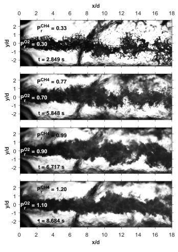
Figure 10: Series of backlit visualizations dynamically showing the evolution of the oxygen from **subcritical** to **transcritical** conditions.
