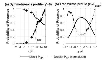
Figure 25: Profiles of  $P_{LP}$  and  $P_{DP}$  sampled along (a) the liquid-jet apparent symmetry axis and (b) its orthogonal axis at the position of the time-averaged breakup (see Figure 24). The profiles of  $P_{DP}$  are normalized by their respective maximum values. The absence of values between the positions marked with "+" symbols corresponds to the non-measurable region imposed by the visualization-window's crack.
