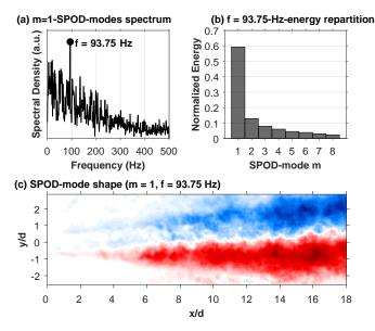
Figure 17: Spectral Proper Orthogonal Decomposition (SPOD) analysis performed on a sequence of OH\* chemiluminescence images within the **Gaseous** Case stabilized plateau. (a) Spectral Density of the most dominant (m = 1) SPOD-modes. (b) Normalized Energy distribution at the f = 93.75-Hzfrequency. (c) Shape of the most dominant SPOD-mode at the f = 93.75-Hz-Hz-frequency.
