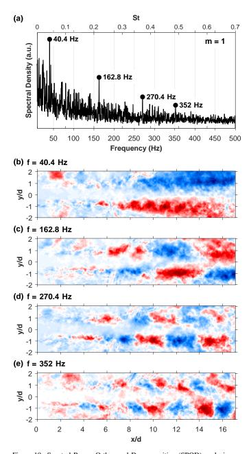
Figure 19: Spectral Proper Orthogonal Decomposition (SPOD) analysis performed on a sequence of backlit images within the **Transcritical** Case stabilized plateau. (a) Spectral Density of the most dominant (m = 1) SPOD-mode. Note that the top horizontal-axis provides values of the oxygen-injection-based Strouhal number,  $\mathbf{St} = fd/U_{O2}$ . (b–e) Shapes of the most dominant SPODmode for the isolated frequencies.
