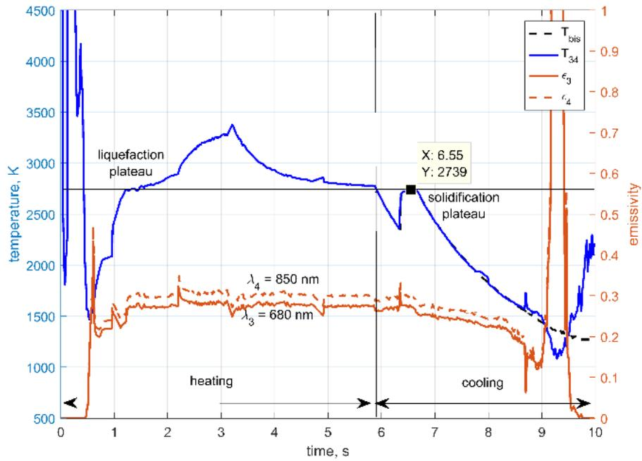
**Figure 9.** Bispectral temperature emissivity estimation for the combination 3/4.
