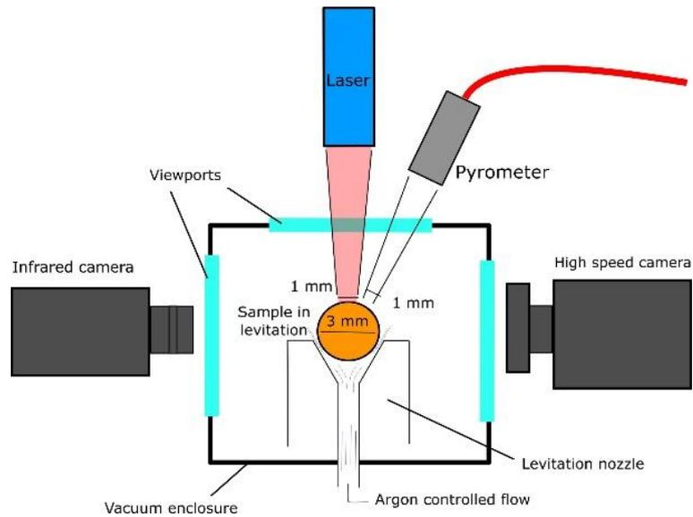
**Figure 1.** Sketch of the aerodynamic levitation apparatus
