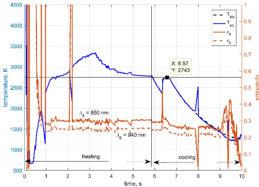
**Figure 10.** Bispectral temperature emissivity estimation for the combination 4/5.
