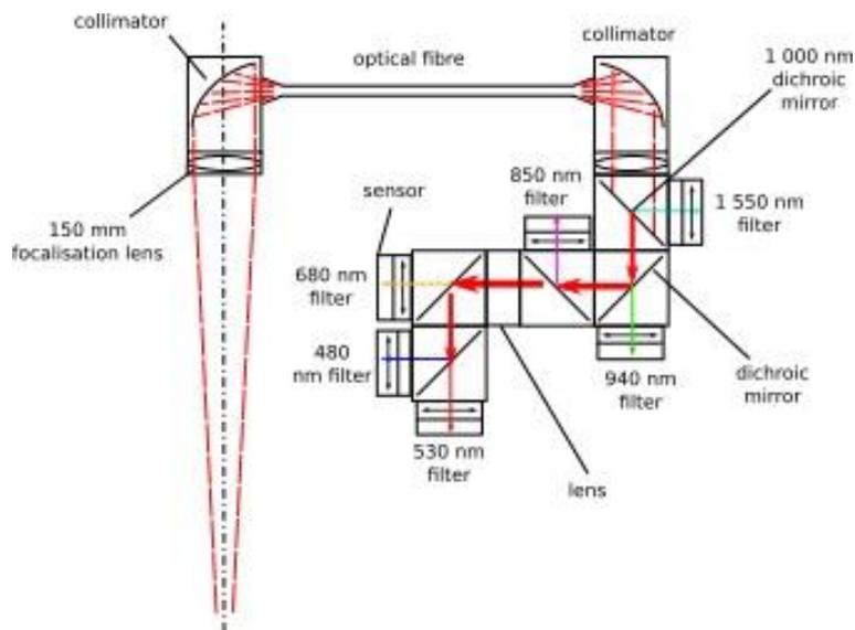
**Figure 2.** Sketch of the six-wavelength pyrometer.
