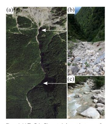
**Figure 1. (a)** The Roize River, a typical mountain stream configuration with **(b)** a production zone with sediment deposits that are several metres thick and show evidence of large incisions and **(c)** a transfer zone consisting of a narrow steep step-pool morphology. Photo credit: **(a)** IGN France (https://www.geoportail.gouv.fr, last access: 16 July 2020).
