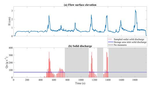
**Figure 6.** In-channel measurement time series of flow surface elevation and solid discharge. Panel (a) shows flow surface elevation as measured in the middle section. Panel (b) shows outlet solid discharge (red bars) compared with inlet solid discharge (blue horizontal line). It is worth recalling that these measurements refer to a different experiment from that presented in Sect. 3.1.
