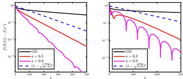
Figure 4: Convergence of QHM. The left plot shows the convergence of 10-dimensional quadratic with  $\mu = 0.01$  and  $L = 1$ ; the right plot reports 10-dimensional regularized logistic regression (random data and labels) with regularization weight  $l = 10^{-4}$ . We specifically used  $s = 0.5$ ,  $\beta = 1 - 2\sqrt{\mu s}$  and  $s = 0.5$ ,  $\beta = 1 - 2\sqrt{l s}$ , respectively, in the two experiments.
