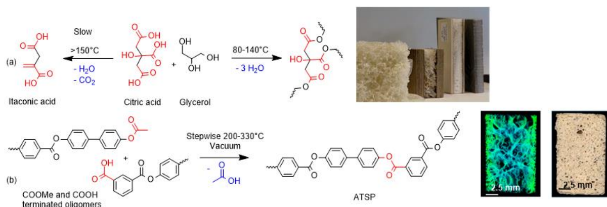
Figure 21: Self-foaming (a) biobased Plantics and (b) aromatic polyesters. (a) is adapted from [223] with permission from the Royal Society of Chemistry, Copyright (2017) and (b) is adapted with permission from [74], Copyright (2016), American Chemical Society.
