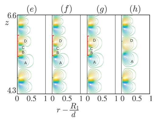
Figure 11: Secondary instability for a Carreau fluid with  $n_c = 0.2$ ,  $\lambda = 200$ , fixed bottom endwall, stress-free at the top endwall at Re = 1.08 Re<sub>c</sub>. Contours of stream function at different times. (a)  $t = T_0$ , (b)  $t = T_0 + 20$ , (c)  $t = T_0 + 49$ , (d)  $t = T_0 + 69$ , (e)  $t = T_0 + 96$ , (f)  $t = T_0 + 110$ , (h)  $t = T_0 + 117$ .
