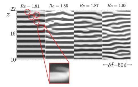
Figure 18: Xanthan gum 2000 ppm,  $n_c=0.34$  and  $\lambda=197$ . Spatio-temporal diagrams at different Reynolds numbers: front view of repetitive creation and merging events. At Re = 1.81,  $50 s = 523 d/(R_1\Omega_1)$ . The insert is a zoom on the emergence of a weakly bright spot in a dark region.
