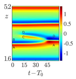
Figure 9: Secondary instability for a Carreau fluid with  $n_c = 0.5$ ,  $\lambda = 200$  at Re =  $1.69 \,\mathrm{Re}_c$ . Periodic boundary conditions in the axial direction with  $\lambda_z = 1.7974$ ,  $L = 7 \,\lambda_z = 12.582$ . Distribution of the azimuthal vorticity along the line  $r = R_1/d + 0.44$  as a function of time: zoom on three pairs of vortices.
