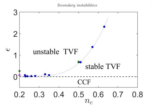
Figure 21: Stability diagram of the TVF regime for a Carreau fluid with  $\eta=0.4$  in the plane ( $\epsilon=(\mathrm{Re}-\mathrm{Re}_c)/\mathrm{Re}_c$ ),  $n_c$ ). The thin dashed line (drawn as a guide for the eye) joins the experimental results represented by filled circles. Numerical results are represented by a filled triangle for realistic boundary conditions and filled diamonds for periodic boundary conditions.
