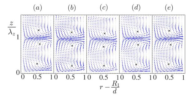
Figure 6: Aqueous glycerol solution. Instantaneous radial-axial velocity vectors in radial-axial plane for wavy vortex flow I at Re = 444 (6.5 Re<sub>c</sub>). The time progresses from left to right through one cycle of an azimuthal wave passing the measurement plane. (a) t = 0, (b)  $t = 5.3 (d/R_1\Omega_1)$ , (c)  $t = 13.25 (d/R_1\Omega_1)$ , (d)  $t = 21.2 (d/R_1\Omega_1)$ , (e)  $t = 26.5 (d/R_1\Omega_1)$ .
