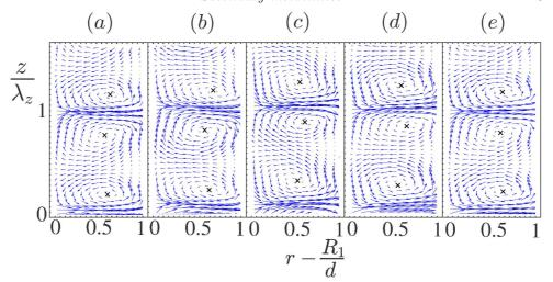
Figure 7: Aqueous glycerol solution. Instantaneous radial-axial velocity vectors in radial-axial plane for wavy vortex flow II at Re = 478 (7 Re<sub>c</sub>). The time progresses from left to right through one cycle of an azimuthal wave passing the measurement plane. (a) t = 0, (b)  $t = 14.4 (d/R_1\Omega_1)$ , (c)  $t = 28.8 (d/R_1\Omega_1)$ , (d)  $t = 43.2 (d/R_1\Omega_1)$ , (e)  $t = 51.8 (d/R_1\Omega_1)$ .
