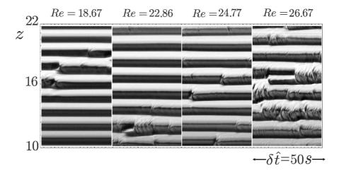
Figure 17: Xanthan gum 1000 ppm,  $n_c = 0.5$  and  $\lambda = 3.1$ . Spatio-temporal diagrams at different Reynolds numbers: front view of repetitive creation and merging events. At Re = 18.67,  $50 s = 342 d/(R_1 \Omega_1)$ .
