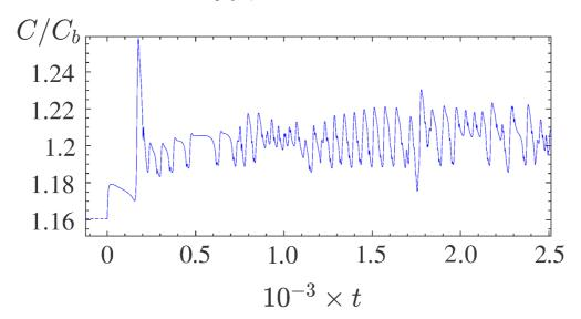
Figure 13: Secondary instability for a Carreau fluid with  $n_c = 0.5$ ,  $\lambda = 200$ . Variation of the ratio of the torque to that obtained for a purely Couette flow with periodic boundary conditions at Re = 1.69 Re<sub>c</sub>. The dashed line before t = 0, is the converged solution at a lower Reynolds number.
