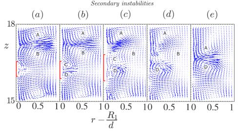
Figure 15: Xanthan gum 1000 ppm with  $n_c = 0.51$ ,  $\lambda = 5.3$ . Velocity field in the plane (r, z). (a)  $\hat{t} = T_0$ , (b)  $\hat{t} = T_0 + 0.2 s = T_0 + 2.1 d/(R_1\Omega_1)$ , (c)  $\hat{t} = T_0 + 1.5 s = T_0 + 1.5 s = T_0 + 1.5 s = T_0 + 1.7 s = T_0$
