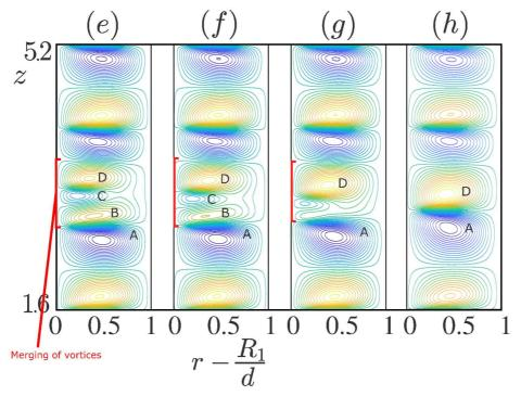
Figure 8: Secondary instability for a Carreau fluid with  $n_c = 0.5$ ,  $\lambda = 200$  at Re =  $1.67\,\mathrm{Re}_c$ . Periodic boundary conditions in the axial direction, with  $\lambda_z = 1.7974$ ,  $L = 7\,\lambda_z = 12.582$ . Contours of stream function at different times: (a)  $t = T_0$ , (b)  $t = T_0 + 6$ , (c)  $t = T_0 + 15$ , (d)  $t = T_0 + 30$ , (e)  $t = T_0 + 36$ , (f)  $t = T_0 + 45$ , (g)  $t = T_0 + 57$ , (h)  $t = T_0 + 64$ .
