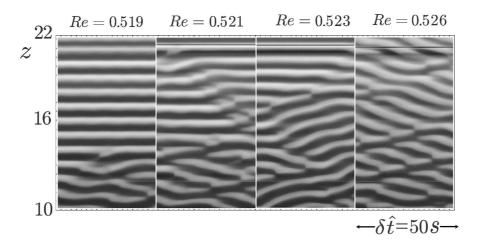
Figure 19: Xanthan gum 3000 ppm,  $n_c=0.23$  and  $\lambda=1255$ . Spatio-temporal diagrams at different Reynolds numbers. At Re = 0.519,  $50 s=809 \, d/(R_1 \Omega_1)$ .
