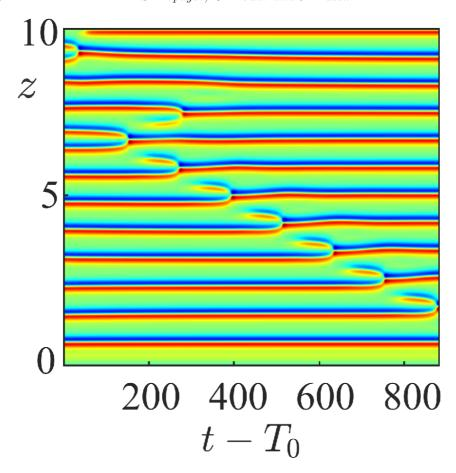
Figure 12: Secondary instability for a Carreau fluid with  $n_c = 0.2$ ,  $\lambda = 200$ , fixed bottom endwall, stress-free at the top, at Re = 1.08 Re<sub>c</sub>. Distribution of the azimuthal vorticity along the line  $r = R_1/d + 0.123$  as a function of time.
