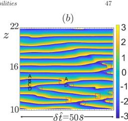
Figure 20: Xanthan gum 3000 ppm,  $n_c = 0.23$  and  $\lambda = 1255$ . Complex demodulation of a spatio-temporal diagram at Re = 0.521: (a) amplitude demodulation dark zones corresponds to the core of the defects where the amplitude vanishes; (b) phase demodulation. Circles and squares show the position of creation and merging processes respectively.
