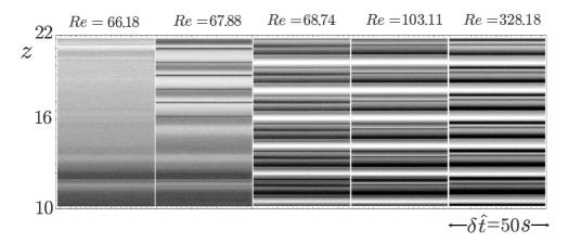
Figure 4: Spatio-temporal diagrams for a 80% by volume of glycerol aqueous solution at Re = 66.18, 67.88, 68.74, 103.11 and Re = 328.18. They are constructed from images taken at 10 frames  $s^{-1}$ . Note that for a Newtonian fluid with  $\eta = 0.4$ , Re<sub>c</sub> = 68.2965. At Re = 66.18,  $50 \text{ s} = 573.05 \, d/(R_1\Omega_1)$
