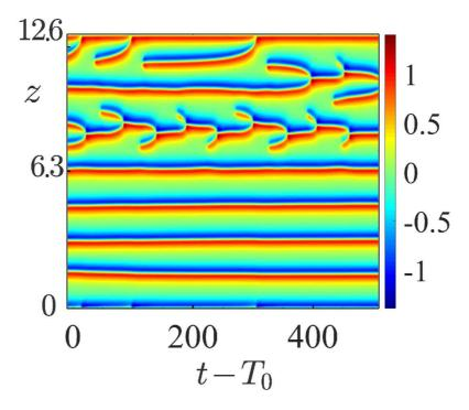
Figure 10: Secondary instability for a Carreau fluid with  $n_c = 0.5$ ,  $\lambda = 200$  at Re =  $1.69\,\mathrm{Re}_c$ . Periodic boundary conditions in the axial direction with  $\lambda_z = 1.7974$ ,  $L = 7\,\lambda_z = 12.582$ . Distribution of the azimuthal vorticity along the line  $r = R_1/d + 0.44$  as a function of time.
