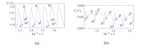
Figure 14: Secondary instability for a Carreau fluid. Variation of the ratio of the torque to that obtained for a purely Couette flow. (a)  $n_c = 0.5$ ,  $\lambda = 200$ , Re = 1.69 Re<sub>c</sub>, periodic boundary conditions in the axial direction. (b)  $n_c = 0.2$ ,  $\lambda = 200$ , Re = 1.08 Re<sub>c</sub>, fixed bottom endwall and stress-free at the top endwall.
