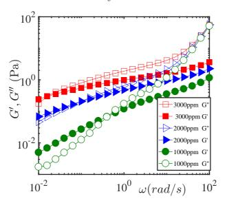
Figure 2: Variation of the elastic G' and viscous G'' as a function of the shear oscillation  $\omega$  for different concentration of xanthan gum solutions.
