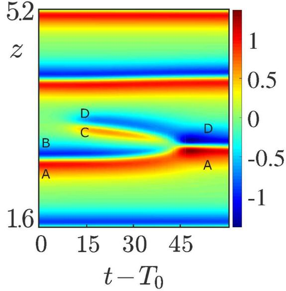
Figure 9: Secondary instability for a Carreau fluid with  $n_c = 0.5$ ,  $\lambda = 200$  at  $\text{Re} = 1.69 \text{Re}_c$ . Periodic boundary conditions in the axial direction with  $\lambda_z = 1.7974$ ,  $L = 7\lambda_z = 12.582$ . Distribution of the azimuthal vorticity along the line  $r = R_1/d + 0.44$  as a function of time: zoom on three pairs of vortices.
