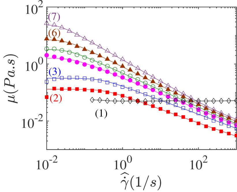
Figure 1: Variation of the viscosity  $\mu$  versus shear rate  $\hat{\gamma}$  for (1) a 80 % by volume glycerol aqueous solution and for aqueous xanthan gum solutions at different concentration. (2) 850 ppm; (3) 1000 ppm; (4) 1200 ppm; (5) 1500 ppm; (6) 2000 ppm and (7) 3000 ppm.
