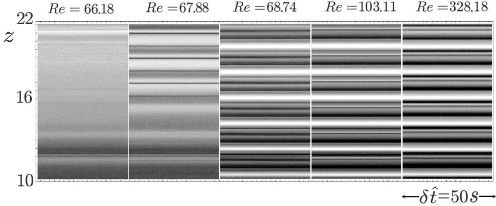
Figure 4: Spatio-temporal diagrams for a 80% by volume of glycerol aqueous solution at  $Re = 66.18, 67.88, 68.74, 103.11$  and  $Re = 328.18$ . They are constructed from images taken at  $10 \text{ frames s}^{-1}$ . Note that for a Newtonian fluid with  $\eta = 0.4$ ,  $Re_c = 68.2965$ . At  $Re = 66.18$ ,  $50 \text{ s} = 573.05 d / (R_1 \Omega_1)$
