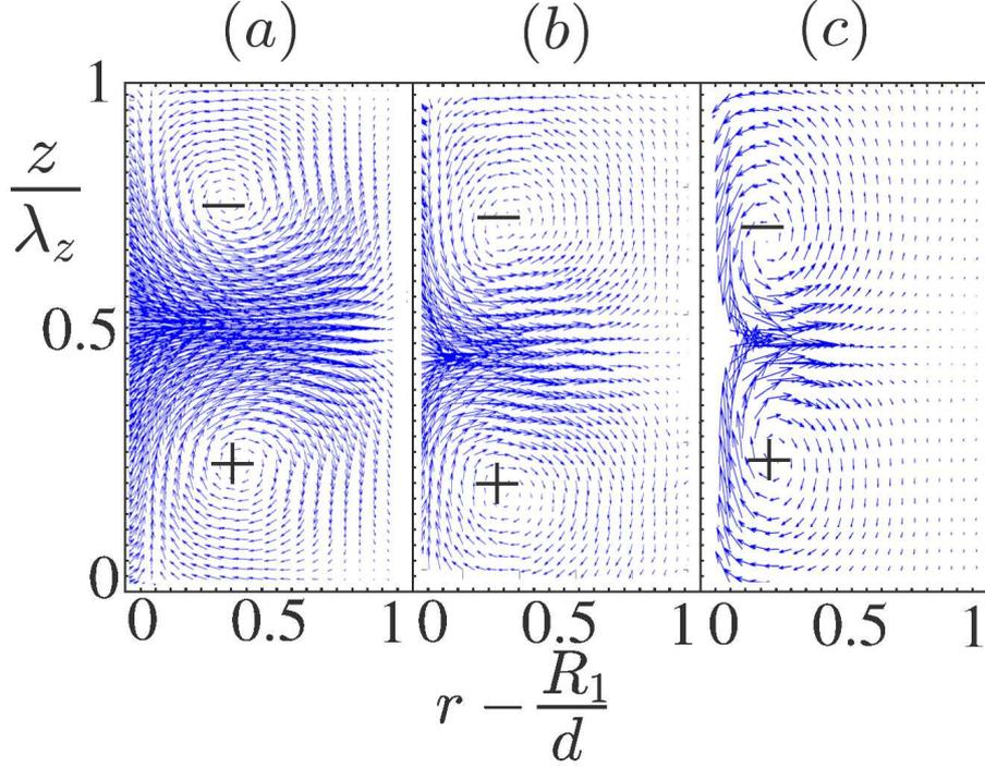
Figure 3: Radial-axial velocity vectors in a radial-axial plane for Taylor vortex flow measured at  $\epsilon \approx 0.01$ . (Left frame) glycerol solution with  $\lambda_z = 2$ ; (middle frame) xanthan gum solution 1000 ppm with  $\lambda_z = 1.8$ ; (right frame) xanthan gum solution 2000 ppm with  $\lambda_z = 1.3$ . For the same length of a vector, the dimensionless velocity in the frames (b) and (c) is two times and four times lower than that in the frame (a), respectively.
