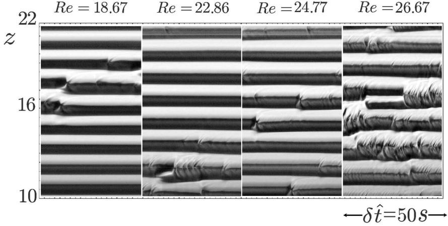
Figure 17: Xanthan gum 1000 ppm,  $n_c = 0.5$  and  $\lambda = 3.1$ . Spatio-temporal diagrams at different Reynolds numbers: front view of repetitive creation and merging events. At  $Re = 18.67$ ,  $50 s = 342d/(R_1\Omega_1)$ .
