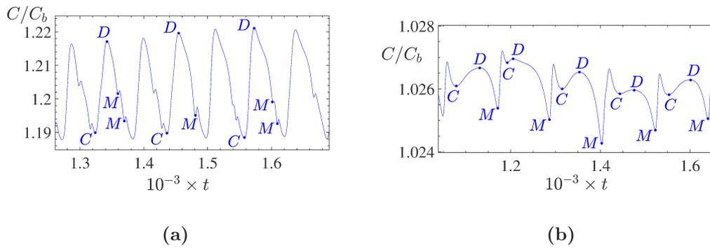
Figure 14: Secondary instability for a Carreau fluid. Variation of the ratio of the torque to that obtained for a purely Couette flow. (a)  $n_c = 0.5$ ,  $\lambda = 200$ ,  $\text{Re} = 1.69 \text{Re}_c$ , periodic boundary conditions in the axial direction. (b)  $n_c = 0.2$ ,  $\lambda = 200$ ,  $\text{Re} = 1.08 \text{Re}_c$ , fixed bottom endwall and stress-free at the top endwall.
