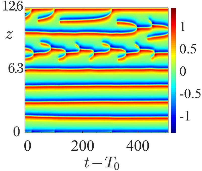
Figure 10: Secondary instability for a Carreau fluid with  $n_c = 0.5$ ,  $\lambda = 200$  at  $\text{Re} = 1.69 \text{Re}_c$ . Periodic boundary conditions in the axial direction with  $\lambda_z = 1.7974$ ,  $L = 7\lambda_z = 12.582$ . Distribution of the azimuthal vorticity along the line  $r = R_1/d + 0.44$  as a function of time.
