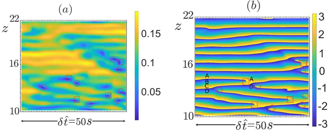
Figure 20: Xanthan gum 3000 ppm,  $n_c = 0.23$  and  $\lambda = 1255$ . Complex demodulation of a spatio-temporal diagram at  $\text{Re} = 0.521$ : **(a)** amplitude demodulation dark zones corresponds to the core of the defects where the amplitude vanishes; **(b)** phase demodulation. Circles and squares show the position of creation and merging processes respectively.
