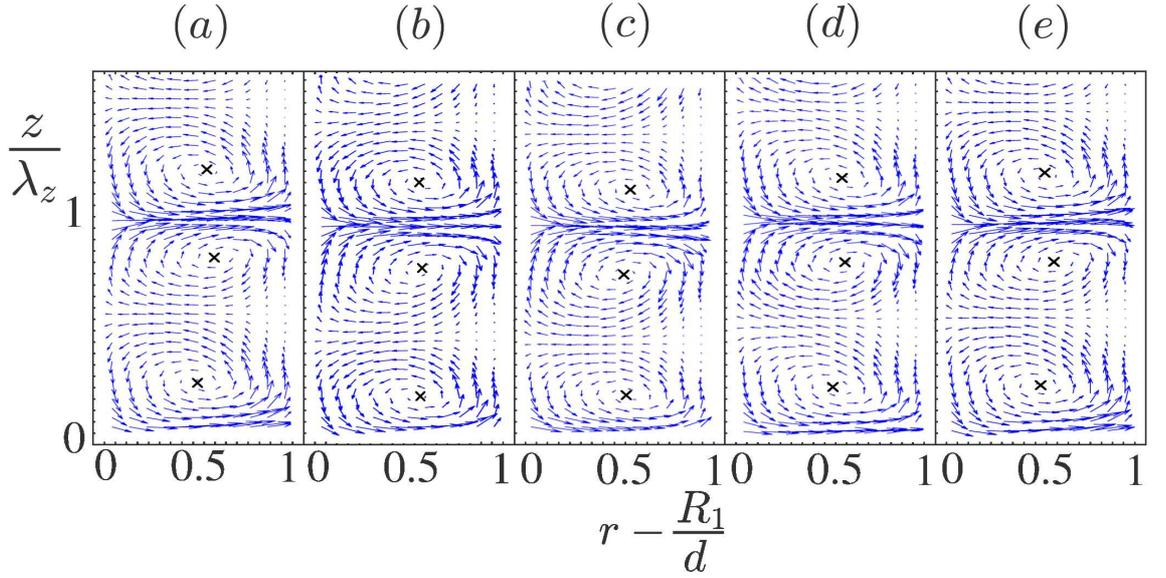
Figure 6: Aqueous glycerol solution. Instantaneous radial-axial velocity vectors in radial-axial plane for wavy vortex flow I at  $\text{Re} = 444 (6.5 \text{Re}_c)$ . The time progresses from left to right through one cycle of an azimuthal wave passing the measurement plane. (a)  $t = 0$ , (b)  $t = 5.3(d/R_1\Omega_1)$ , (c)  $t = 13.25(d/R_1\Omega_1)$ , (d)  $t = 21.2(d/R_1\Omega_1)$ , (e)  $t = 26.5(d/R_1\Omega_1)$ .
