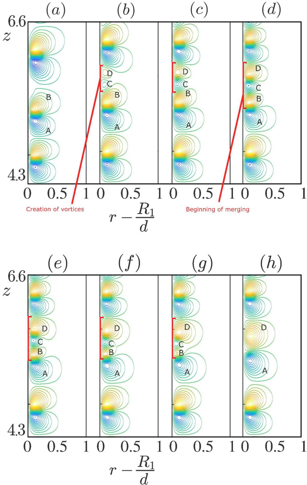
Figure 11: Secondary instability for a Carreau fluid with  $n_c = 0.2$ ,  $\lambda = 200$ , fixed bottom endwall, stress-free at the top endwall at  $Re = 1.08 Re_c$ . Contours of stream function at different times. (a)  $t = T_0$ , (b)  $t = T_0 + 20$ , (c)  $t = T_0 + 49$ , (d)  $t = T_0 + 69$ , (e)  $t = T_0 + 96$ , (f)  $t =$ , (g)  $t = T_0 + 110$ , (h)  $t = T_0 + 117$ .
