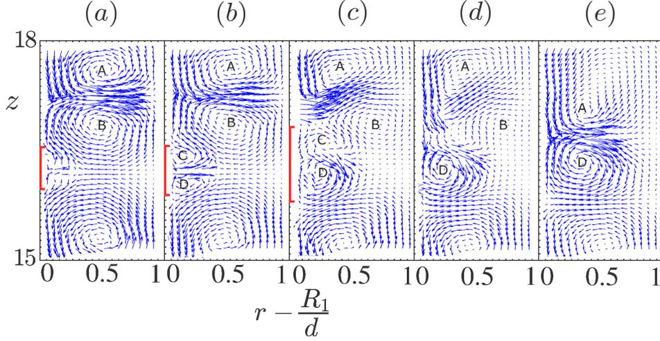
Figure 15: Xanthan gum 1000 ppm with  $n_c = 0.51$ ,  $\lambda = 5.3$ . Velocity field in the plane  $(r, z)$ . (a)  $\hat{t} = T_0$ , (b)  $\hat{t} = T_0 + 0.2 s = T_0 + 2.1 d/(R_1\Omega_1)$ , (c)  $\hat{t} = T_0 + 1.5 s = T_0 + 15.8 d/(R_1\Omega_1)$ , (d)  $\hat{t} = T_0 + 1.7 s = T_0 + 17.9 d/(R_1\Omega_1)$ , (e)  $\hat{t} = T_0 + 2 s = T_0 + 21 d/(R_1\Omega_1)$ .
