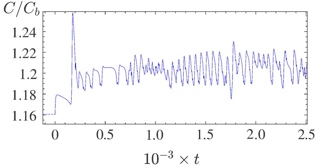
Figure 13: Secondary instability for a Carreau fluid with  $n_c = 0.5$ ,  $\lambda = 200$ . Variation of the ratio of the torque to that obtained for a purely Couette flow with periodic boundary conditions at  $\text{Re} = 1.69 \text{Re}_c$ . The dashed line before  $t = 0$ , is the converged solution at a lower Reynolds number.
