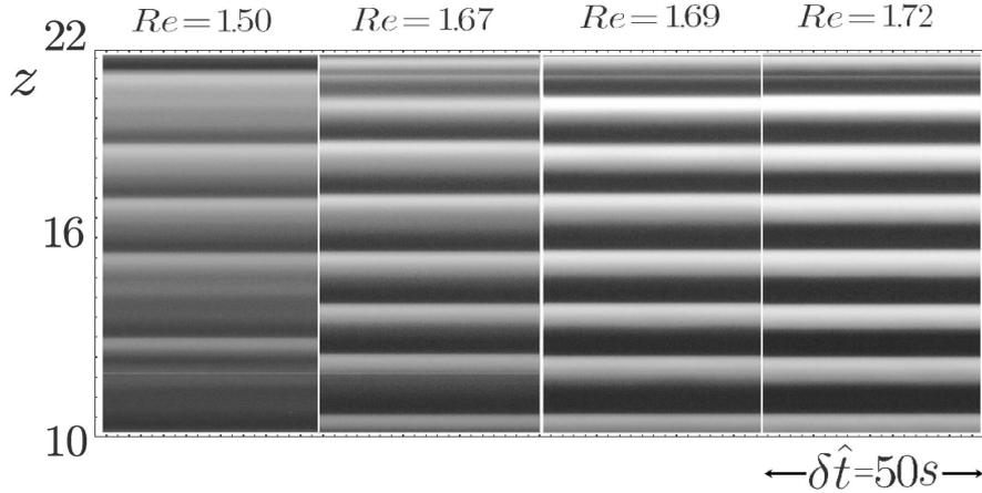
Figure 5: Space-time diagrams of xanthan gum 2000 ppm for  $Re = 1.5, 1.67, 1.69$  and  $1.72$ . The rheological parameters are  $n_c = 0.34$ ,  $\lambda = 197$ . For this case, the linear theory gives  $Re_c = 1.6944$ . At  $Re = 1.5$ ,  $50 \text{ s} = 1099 d / (R_1 \Omega_1)$
