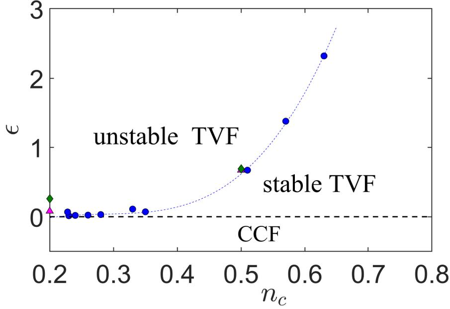
Figure 21: Stability diagram of the TVF regime for a Carreau fluid with  $\eta = 0.4$  in the plane  $(\epsilon = (\text{Re} - \text{Re}_c)/\text{Re}_c, n_c)$ . The thin dashed line (drawn as a guide for the eye) joins the experimental results represented by filled circles. Numerical results are represented by a filled triangle for realistic boundary conditions and filled diamonds for periodic boundary conditions.
