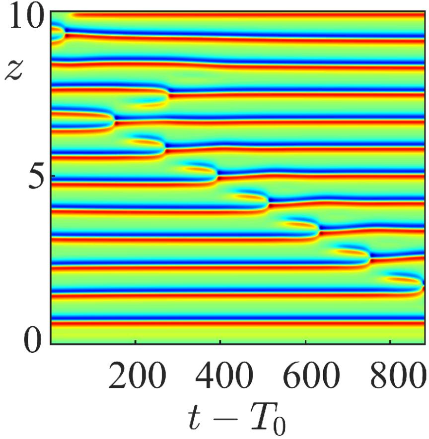
Figure 12: Secondary instability for a Carreau fluid with  $n_c = 0.2$ ,  $\lambda = 200$ , fixed bottom endwall, stress-free at the top, at  $Re = 1.08 Re_c$ . Distribution of the azimuthal vorticity along the line  $r = R_1/d + 0.123$  as a function of time.
