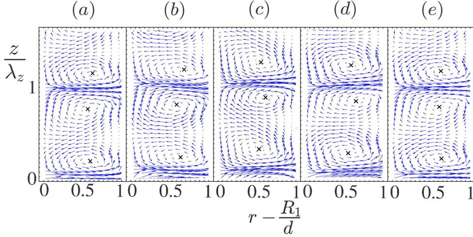
Figure 7: Aqueous glycerol solution. Instantaneous radial-axial velocity vectors in radial-axial plane for wavy vortex flow II at  $Re = 478$  ( $7 Re_c$ ). The time progresses from left to right through one cycle of an azimuthal wave passing the measurement plane. (a)  $t = 0$ , (b)  $t = 14.4(d/R_1\Omega_1)$ , (c)  $t = 28.8(d/R_1\Omega_1)$ , (d)  $t = 43.2(d/R_1\Omega_1)$ , (e)  $t = 51.8(d/R_1\Omega_1)$ .
