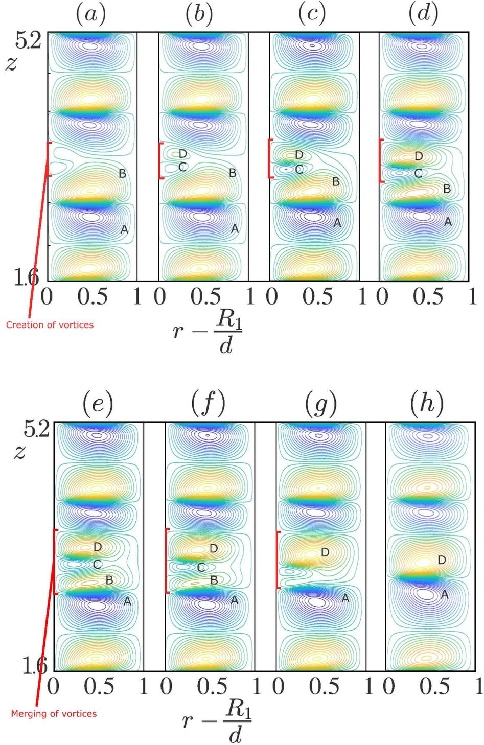
Figure 8: Secondary instability for a Carreau fluid with  $n_c = 0.5$ ,  $\lambda = 200$  at  $\text{Re} = 1.67 \text{Re}_c$ . Periodic boundary conditions in the axial direction, with  $\lambda_z = 1.7974$ ,  $L = 7\lambda_z = 12.582$ . Contours of stream function at different times: (a)  $t = T_0$ , (b)  $t = T_0 + 6$ , (c)  $t = T_0 + 15$ , (d)  $t = T_0 + 30$ , (e)  $t = T_0 + 36$ , (f)  $t = T_0 + 45$ , (g)  $t = T_0 + 57$ , (h)  $t = T_0 + 64$ .
