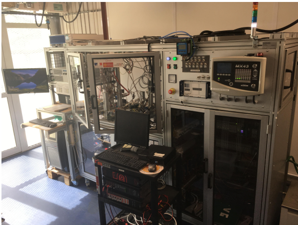
Figure 1. Aging test-bench for start-up & shut-down cycling.
