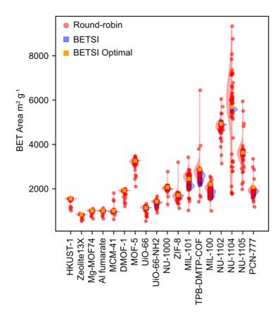
**Figure 1 | Round-robin results and BETSI results.** Distribution of BET areas from identical isotherms as calculated by 60 laboratories with expertise in adsorption science and synthesis of porous materials in red. Superimposed are normalised probability distribution functions obtained by kernel density estimation. Predictions under BETSI are shown in blue alongside, and the 'optimal' BET area in yellow.
