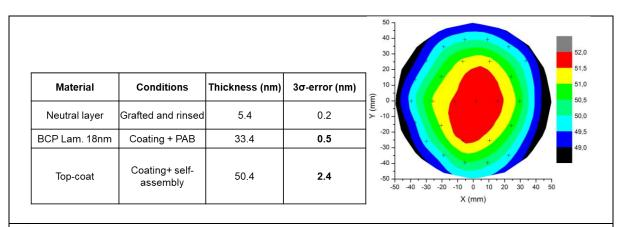
**Figure 3**: Thickness variations observed in 4 inches wafers of the different materials involved in the stack for the self-assembly process, showing a good coating uniformity for all the layers, even after the self-assembly annealing step performed; 31 points of measurement performed for each layer (left). Ellipsometry map of the 31 measurements points highlighting the good uniformity of the TC layer (right).
