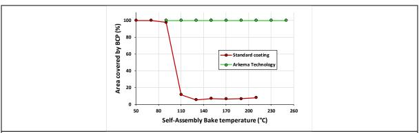
**Figure 5**: Dewetting experiment comparing Arkema's TC technology with a standard neutral TC. The standard coating does not prevent the dewetting of the BCP, while the Arkema's dedicated chemistry one is able to maintain the planarity of the stack even at very high self-assembly temperatures.
