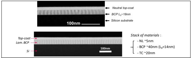
**Figure 4**: FIB-STEM cross-section obtained for typical samples of lamellar BCP PDMSB-*b*-PS with period of 18 nm (top) and 14 nm (bottom), showing perpendicular features across the whole film-thickness. PDMSB-phase appears in dark-grey color, while PS-phase is in light-grey in the corresponding BCP layer.
