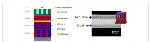
**Figure 6**: Potential tunable parameters in an hypothetical stack of BCPs to obtain different final properties (left). Example of stack of cylindrical BCP buried underneath a perpendicular lamellar BCP owing to Arkema's TC technology, enabling the stack to be ready in less than 10 minutes (self-assembly bake performed at 240°C-5minutes) (right).
