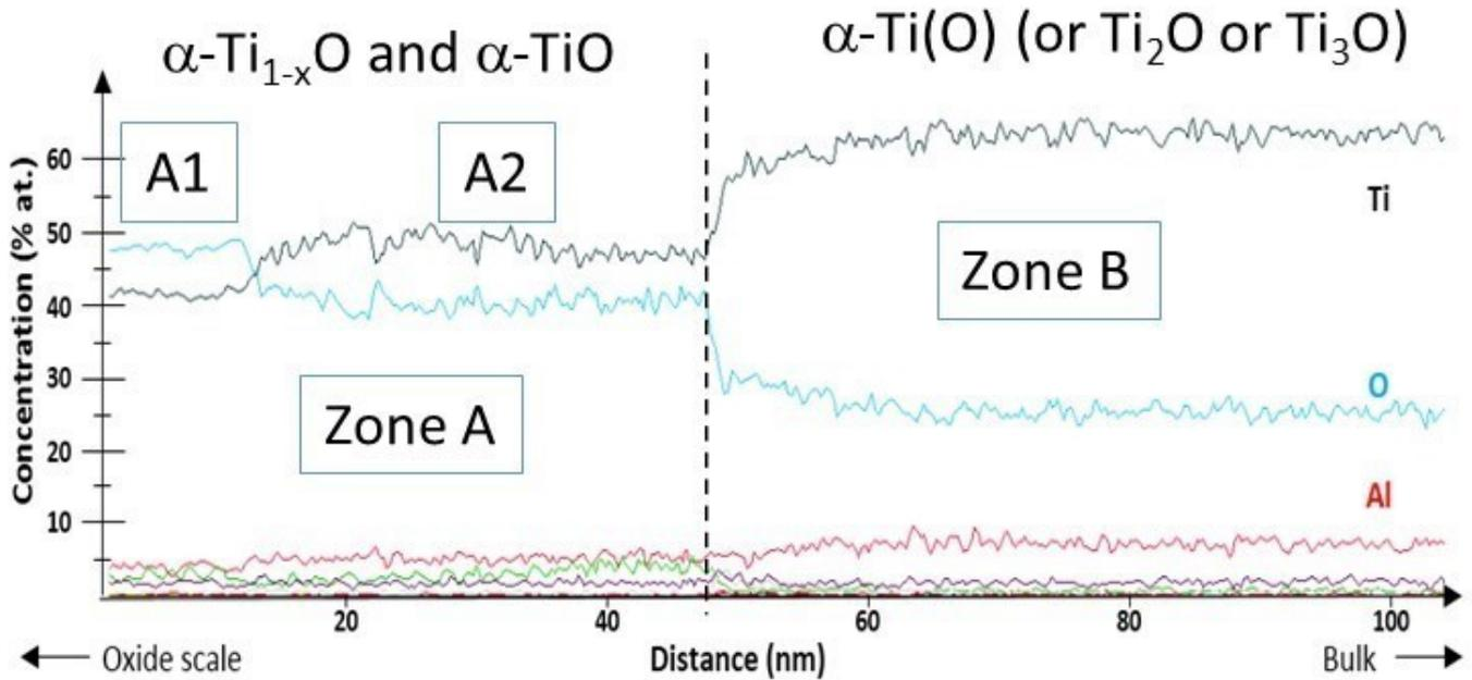
Figure 6: Concentration profiles in one micro-tip analysed by APT after oxidation at 650 °C for 1000 h in Ar-20%O<sub>2</sub>
