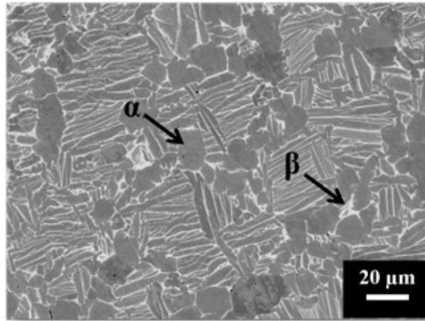
Figure 1: SEM observation of Ti6242S microstructure (BSE mode)
