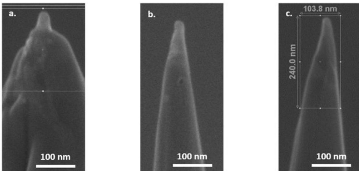
Figure 5: SEM-FEG (Secondary Electron mode) observations of micro-tips obtained by FIB and analysed by APT for Ti6242S oxidized 1000 h at 650 °C in a. Ar-20%O<sub>2</sub>, b. and c. synthetic air
