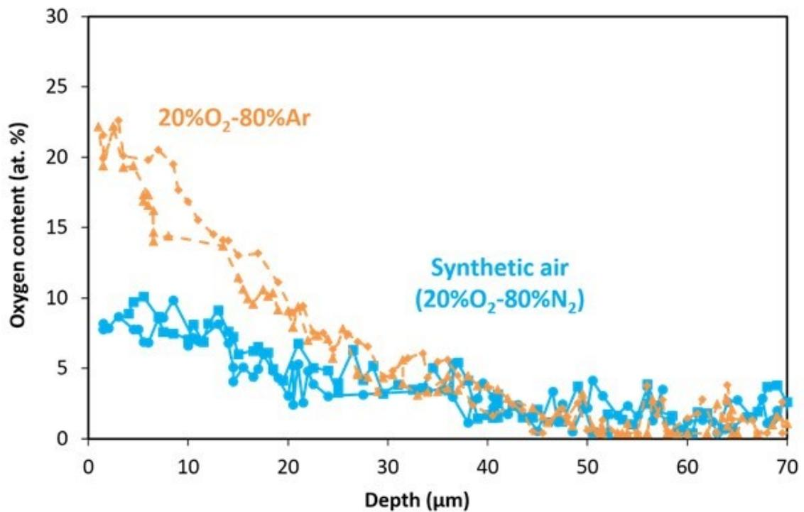
Figure 3: EPMA profiles for oxygen for Ti6242S oxidized at 650 °C for 1000 h in synthetic air (squares, circles and continuous lines) and 20%O<sub>2</sub>-80%Ar (triangles, diamonds and dashed lines)
