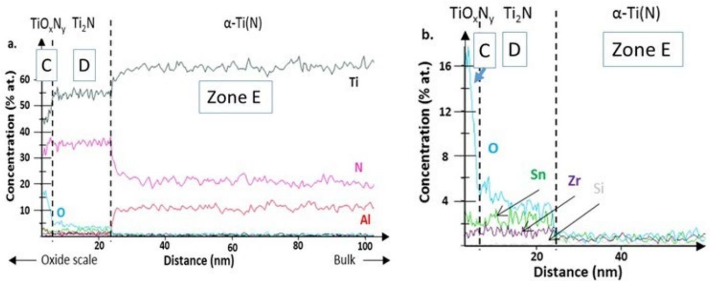
Figure 7: Concentration profiles in one micro-tip analysed by APT after oxidation at 650 °C for 1000 h in synthetic air a. global and b. enlargement for the 60 first nanometres
