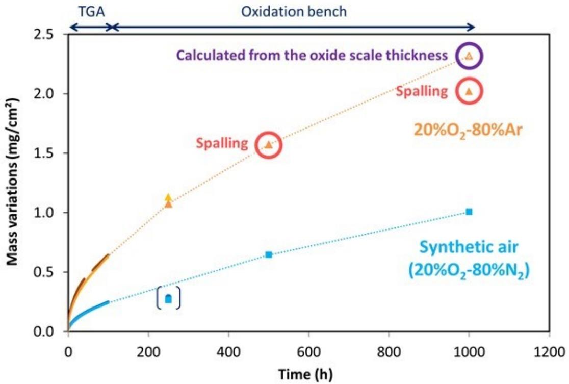
Figure 2: Mass variation vs time for Ti6242S alloy oxidized at 650 °C in flowing synthetic air and Ar-20%O<sub>2</sub> gas mixture
