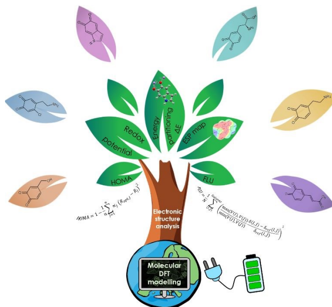
Figure 1. Illustration of the strategy, specific tools and type of materials considered in this work, encompassing: i) molecular electrostatic surface potential (ESP) maps to identify the preferred potential location of metal-ions ii) electron delocalization indices ( i.e. the Harmonic Oscillator Model of Aromaticity (HOMA) and Aromatic Fluctuation index (FLU) descriptors) to account for the variation of the quinoidic ring stability as a function of reduction stage, along with iii) the partitioning of the global energy of the molecule into atomic or atomic group energy contributions, which leaves the possibility to shed light on the predominant role played by some moieties on the global stabilization/destabilization features or to account for the balance between some competitive effects and finally iv) net atomic charges able to give indication either on charge transfers or on electrostatic interactions.
