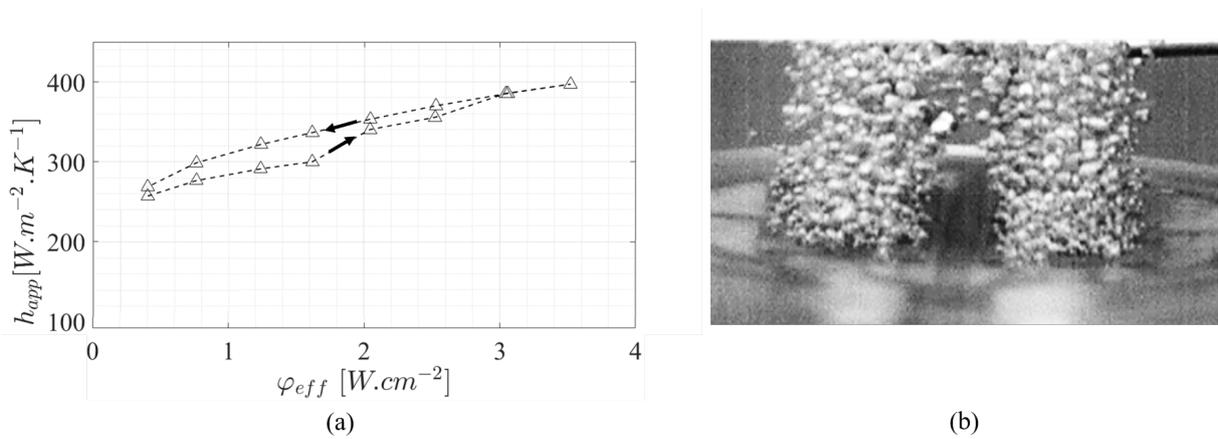
Figure 5: Thermal measurements: (a) Apparent heat transfer coefficient as a function of the effective heat flux density, (b) Nucleate boiling visualization on the polymer evaporator,  $\phi_{eff} = 3.5 \text{ W.cm}^{-2}$ .
