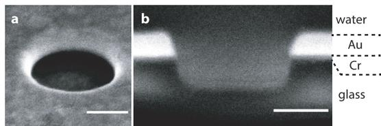
**FIG. 7.** Scanning electron microscope images of an experimental 300 nm diameter nanohole etched using focus ion beam on a 100 nm thick gold layer. (a) Tilted view and (b) cross section. The chromium adhesion layer is clearly visible as a thin gray layer between the gold layer (white) and the glass substrate (black). Scale bars: 150 nm. Courtesy of Jean-Benoit Claude and Jerome Wenger.
