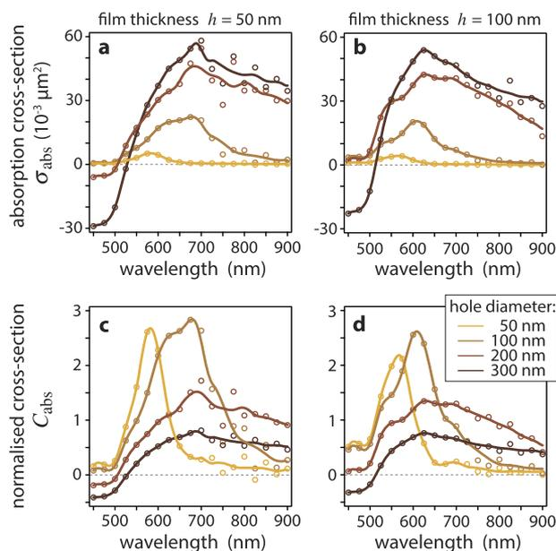
**FIG. 9.** (a) Absorption cross sections of nanoholes with diameters ranging from 50 to 300 nm in a 50-nm thick gold layer. (b) Same as (a) for a 100-nm thick gold layer. (c) and (d) Same as (a) and (b) where the cross sections have been normalized by the area of the nanohole.
