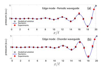
FIG. 11. (a) The edge mode profile corresponding to the experimental setup as obtained by the analytical solution (squares), numerical simulations (solid line) and experiments (circles). (b) The same as (a) but for the case of a disorder realization.
