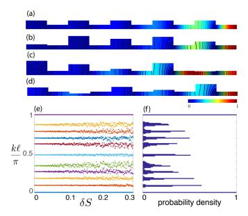
FIG. 8. (a) The edge mode in the periodic case (without disorder). [(b)–(d)] The edge modes for three different disorder realizations of strength  $\delta S = 0.3$  as obtained numerically. (e) The eigenfrequency spectrum of a disorder realization as a function of the disorder strength  $\delta S$ . (f) The probability density of the eigenvalues for a set of  $10^3$  disorder realizations.
