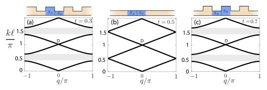
FIG. 2. The dispersion relation of the acoustic SSH for three different values of the coupling t = 0.3 (a), t = 0.5 (b), t = 0.7 (c). This illustrates the band inversion of the model. The crossing of the two bands of the SSH model at s = t appears exactly for the simple waveguide with constant cross section as shown in panel (b).
