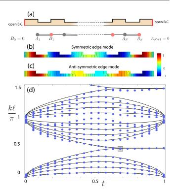
FIG. 3. Open boundary conditions and even cross section changes. (a) Schematic representation of the waveguide configuration with open boundary conditions and the lattice model corresponding to the one-dimensional limit of the waveguide. The symmetric (b) and antisymmetric (c) edge modes as obtained numerically for a waveguide with 2N + 1 = 11 and t = 2/3. (d) The spectrum of the same waveguide of 2N + 1 = 11 segments as a function of t.
