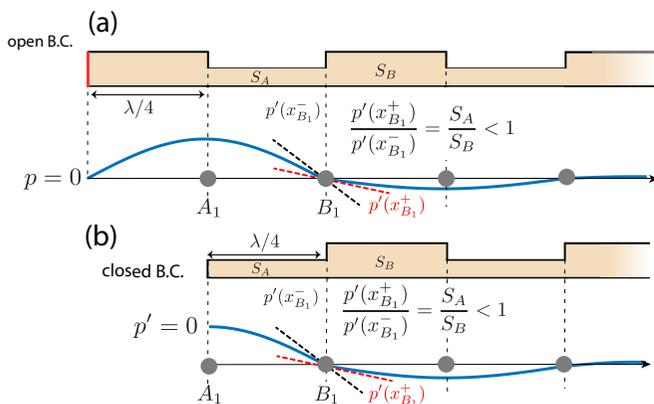
FIG. 6. Graphical construction of the edge modes corresponding to the case of open (a) and closed (b) boundary conditions. The dashed lines at point  $B_1$  illustrate the reduction of slope and thus of the oscillation amplitude.
