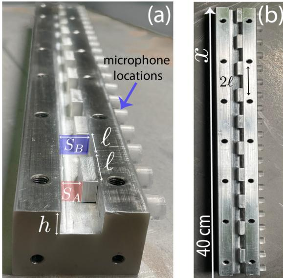
FIG. 9. Experimental setup. (a) Side view of the waveguide where the two different cross sections are indicated. Cross section changes appear every  $\ell$ . In (b) we show the whole waveguide of total length 40 cm, which is composed of  $N = 10$  unit cells.
