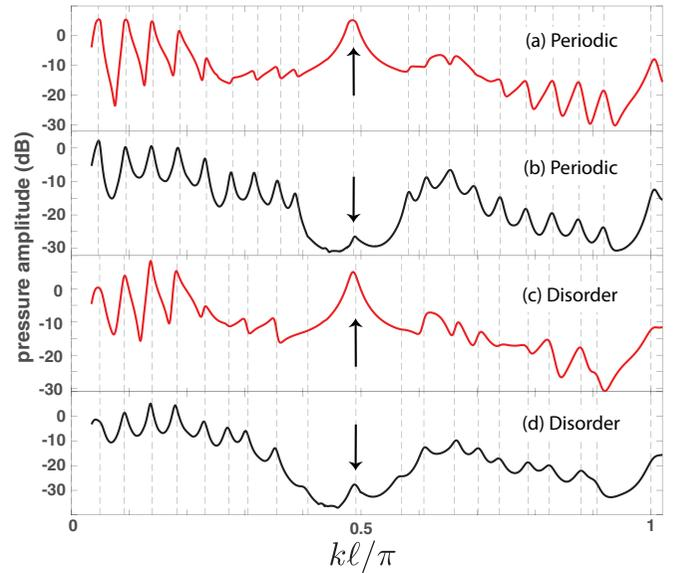
FIG. 10. (a) Pressure amplitude as a function of frequency for a periodic SSH configuration with  $t = 0.63$  measured at 4 cm from the source. (b) Same as panel (a) but the pressure amplitude is obtained using the mean value of the measured pressure at all the junctions. The dashed vertical lines indicate the frequency of the modes as obtained numerically. [(c),(d)] Same as panel [(a),(b)] for a disordered configuration with a mean value  $\langle t \rangle = 0.63$ .
