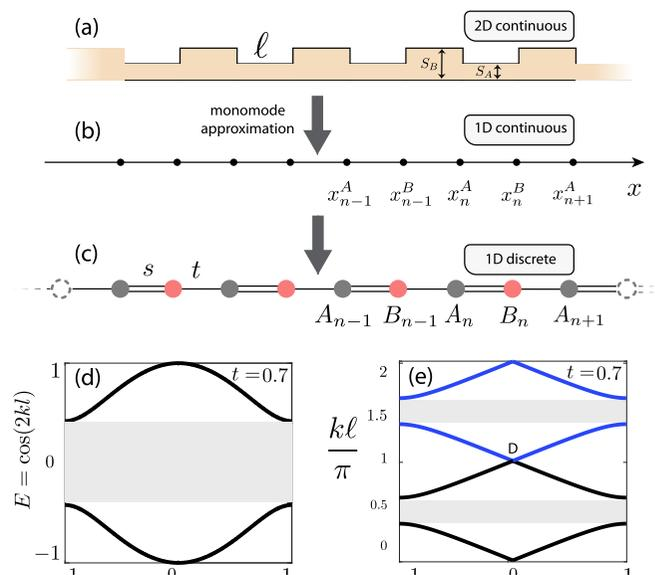
FIG. 1. (a) A sketch of a 2D acoustic waveguide composed of segments of the same length  $\ell$  and different cross sections  $S_A$  and  $S_B$ . (b) Under the monomode approximation the acoustic pressure depends only on the axial coordinate  $x$ . On this axis, we can identify the points where the cross sections change. (c) The explicit map onto the SSH discrete model. [(d),(e)] The dispersion relation of the SSH model as given by Eq. (15).
