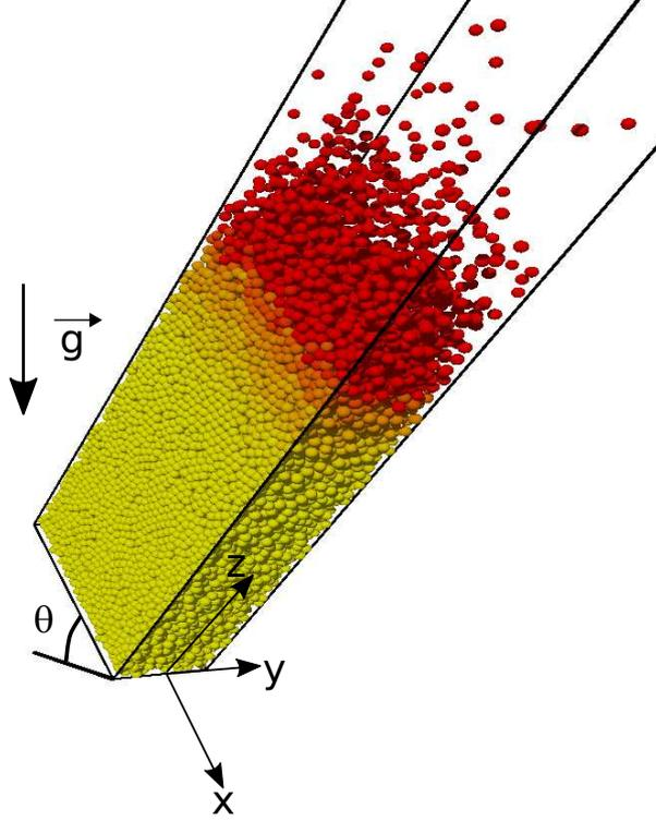
**Figure 1.** Typical snapshot for SSH flows:  $W/d = 10$  and  $N = 15,000$ . The angle of the flow is  $\theta = 45^\circ$ , the coefficient of restitution  $e_n$  is equal to 0.88, and the grain-grain and grains-wall friction coefficients (respectively  $f_g$  and  $f_w$ ) are set to 0.5. Flow is directed down the incline along the  $x$ -axis. Two sidewalls confining the system are parallel to the  $(xz)$  plane.
