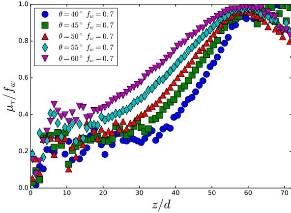
**Figure 3.** The effective friction coefficient on sidewalls,  $\mu_\tau$ , is strongly influenced by confinement. In the vicinity of the free surface, it is close to the grain-sidewall friction coefficient,  $f_w$ . Then, it weakens and, in the creep zone, reaches a constant value.
