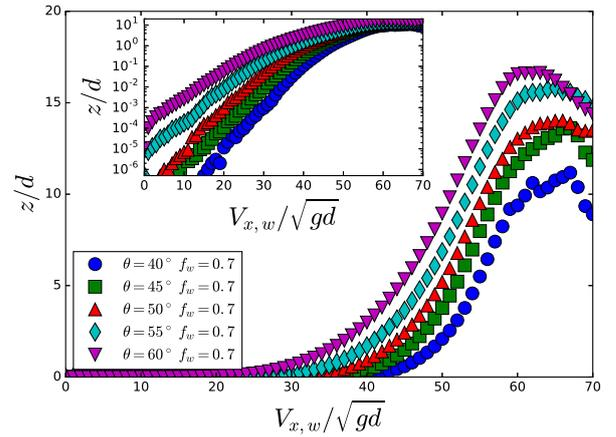
**Figure 2.** The velocity in the streamwise direction and at sidewalls,  $V_{x,w}$  increases with flow angle and displays an exponential variation characteristic of creeping in the vicinity of the bottom (inset).
