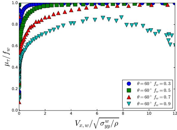
**Figure 5.** Zhu’s relation (ratio of the effective friction coefficient at sidewalls to the microscopic grain-sidewall friction coefficient versus the Froude number at sidewalls  $V_{x,w} / \sqrt{\sigma_{xx}^w / \rho}$ ) is found to depend on the grain-sidewall microscopic friction coefficient.
