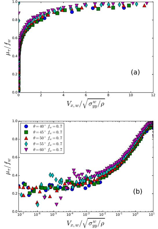
**Figure 4.** For a given system, the relation between the effective sidewall friction coefficient  $\mu_\tau$  and the Froude number at sidewalls is unique (a). This is true even at small Froude numbers (b).
