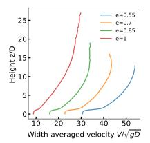
Figure 6: Vertical velocity profiles for decreasing restitution coefficient. The inclination angle is  $\theta = 40^{\circ}$  and the particle hold-up is H = 5D.
