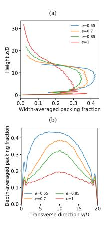
Figure 5: (a) Vertical packing fraction profiles for decreasing restitution coefficient. (b) Corresponding transverse packing fraction profiles. The inclination angle is  $\theta = 40^{\circ}$ and the particle hold-up is H = 5D.
