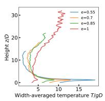
Figure 7: Vertical temperature profiles for decreasing restitution coefficient. The inclination angle is  $\theta = 40^{\circ}$  and the particle hold-up is H = 5D.
