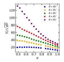
Figure 3: Mean flow velocity as a function of the restitution coefficient for various values of the inclination angle. The particle hold-up is H = 5D.
