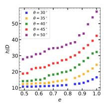
Figure 4: Flow height *h* as a function of the restitution coefficient for various values of the inclination angle. The particle hold-up is H = 5D.
