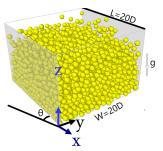
Figure 1: Flow geometry: The granular flow is confined by lateral walls with a width W = 20D. Periodic boundary conditions are used in the stream-wise direction with a length L and an angle of inclination  $\theta$ .
