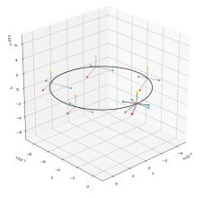
Figure 5: Trajectory of SPR4 associated with the optimal control curve realizing a net displacement proportional to  $\delta p_2$ , i.e. a rotation around the z-axis. The initial and final positions are marked by neon green and purple arms, respectively.
