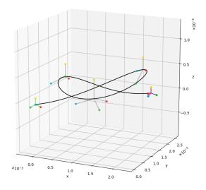
Figure 6: Trajectory of SPR4 associated with the optimal control curve realizing a net displacement proportional to  $\delta p = (2, 2, 0, 0, 0, 1)$ . The initial and final positions are marked by neon green and purple arms, respectively.
