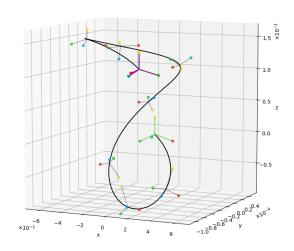
Figure 7: Trajectory of SPR4 associated with the optimal control curve realizing a net displacement proportional to  $\delta p_4$ , i.e. a screw motion along the z-axis. The initial and final positions are marked by neon green and purple arms, respectively.
