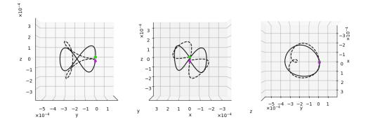
Figure 8: A case of non-unique optimal trajectories. Two trajectories are shown yielding to the same displacement and rotation  $\delta p$  such that  $\Lambda^{-1}\delta p \sim \tau_1 \wedge \tau_2 + \tau_3 \wedge \tau_4$ , one in solid line, and the other in dotted line. The three picture correspond respectively to the front, side and top views of those two trajectories.
