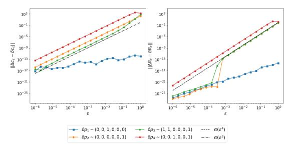
Figure 3: The numerical convergence behavior of the theoretical net displacement in Proposition 5 in both translation and rotation.
