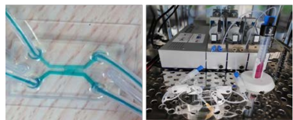
Figure 2: (top) Schematic of the microfluidic system and description of its implementation as a 3D dynamic culture reactor for PC model; (bottom-left) Actual device made of PDMS & glass and dynamically perfused with blue colored water; (bottom-right) Photo of the device connected to the syringe pump and culture medium reservoir in the incubation chamber.
