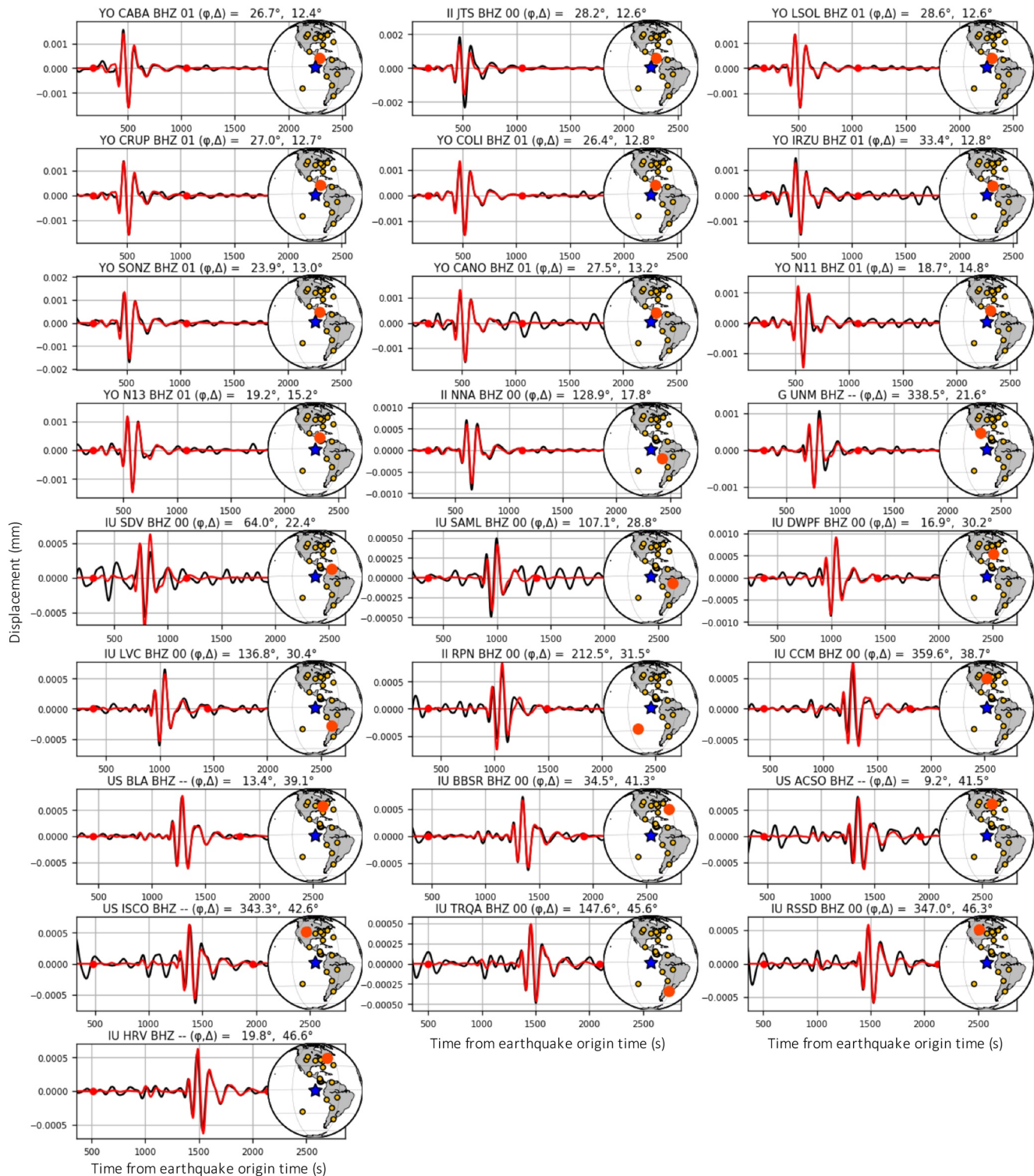
Figure 6. Model performance of MT inversion for the M_w 5.5 vertical-T CLVD earthquake of October 22, 2005. Red and black lines represent synthetic and observed waveforms, respectively. The start and end points of the inversion time window are indicated by red circles. In each inset map, the blue star and the large red circle represent locations of the epicenter ( 0.83^\circ\text{S} , 91.14^\circ\text{W} ) and the station. The station azimuth ( \phi ) and epicentral distance ( \Delta ) are indicated at the top of each panel.
