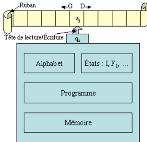
Figure 10. Schéma de la machine de Turing. URL: [http://www.desmontils.net/emiage/Module209EMiage/c5/Ch5\\_2.htm](http://www.desmontils.net/emiage/Module209EMiage/c5/Ch5_2.htm)
