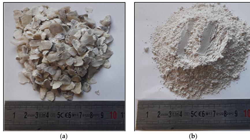
**Figure 1.** Oyster shells. (a) before grinding; (b) after grinding.
