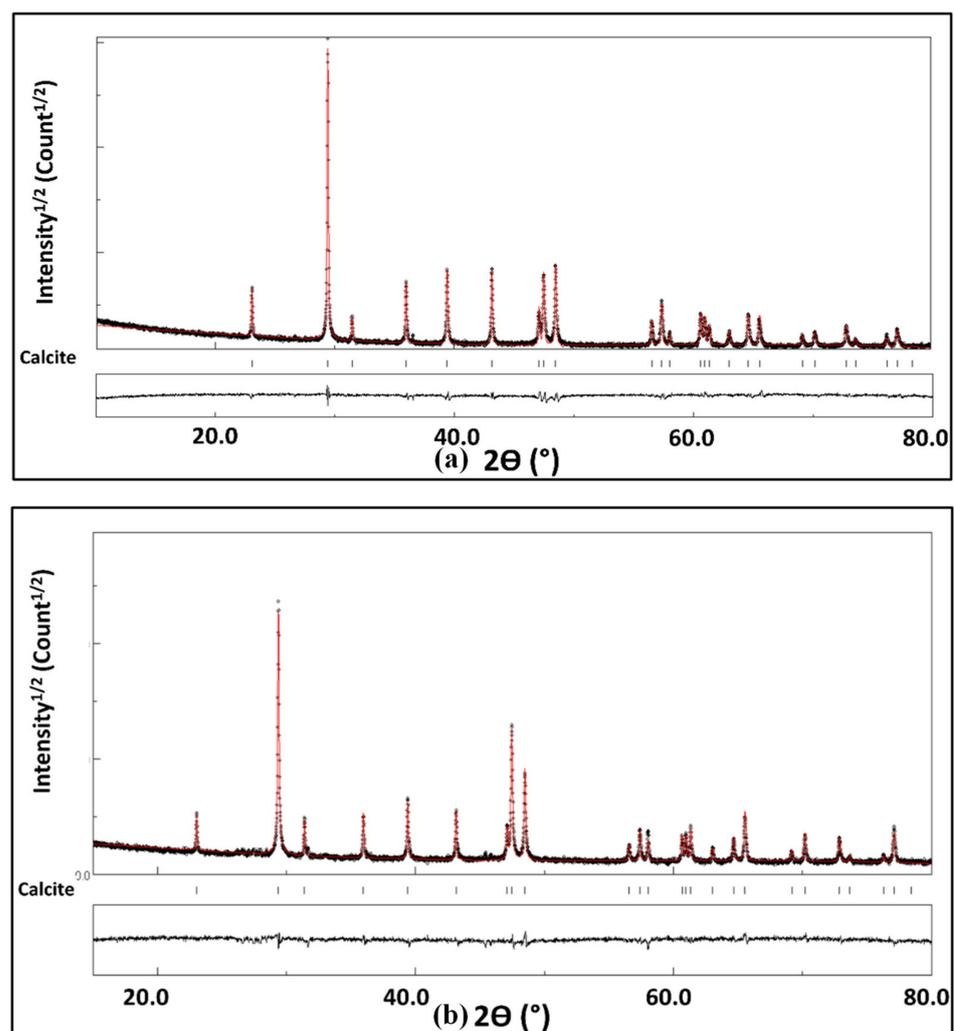
**Figure 8.** X-ray diffraction patterns of (a) LF and (b) GOS refined using the MAUD software. The calculated pattern (red line) is superimposed on the observed profile (coarse line). The difference curve ( $I_{obs} - I_{calc}$ ) is shown at the bottom.
