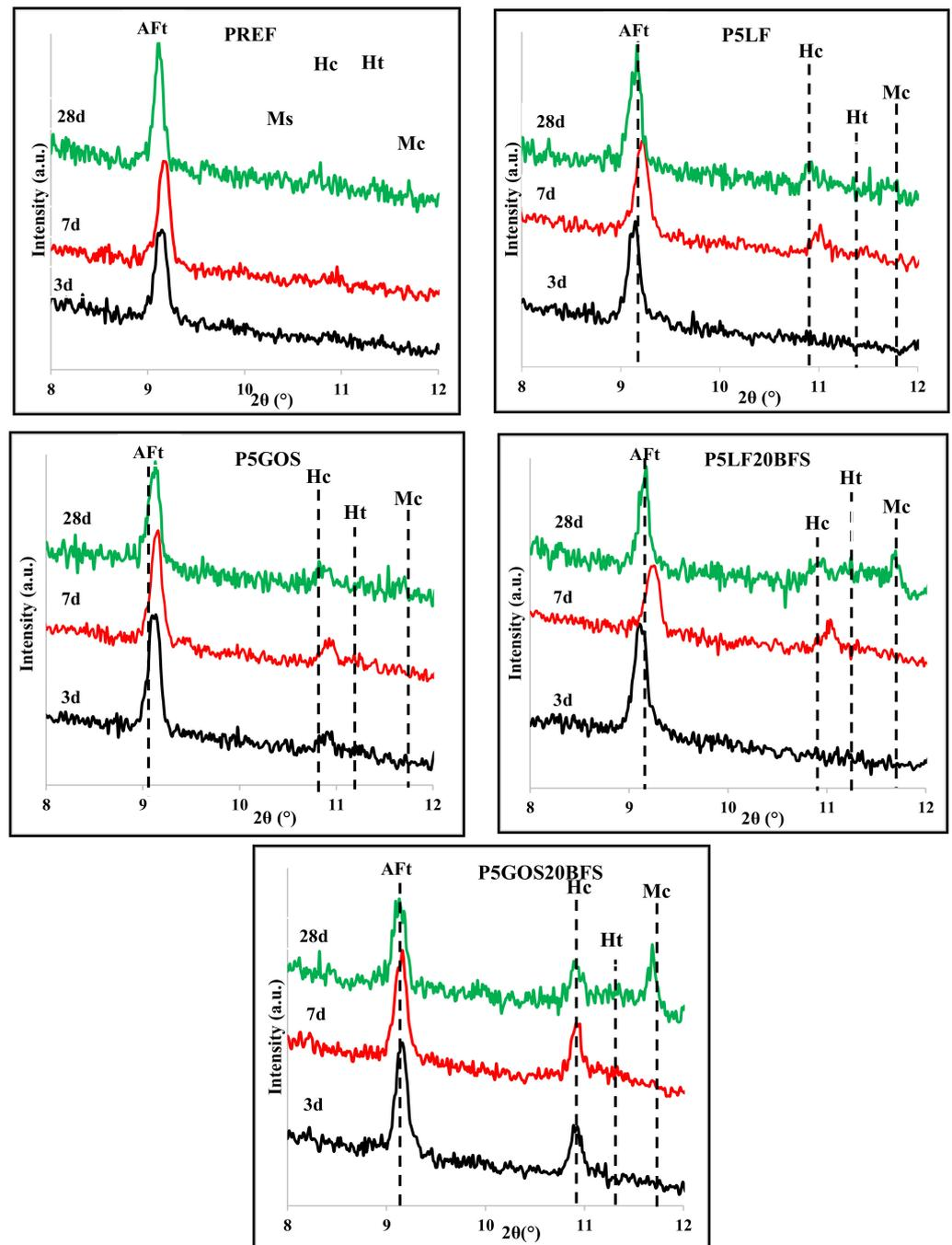
**Figure 3.** XRD patterns and identified phases within  $2\theta$  range of 5–12 °C for binary and ternary cement pastes studied. Aft-ettringite, Hc- Hemicarboaluminate, Mc-monocarboaluminate.
