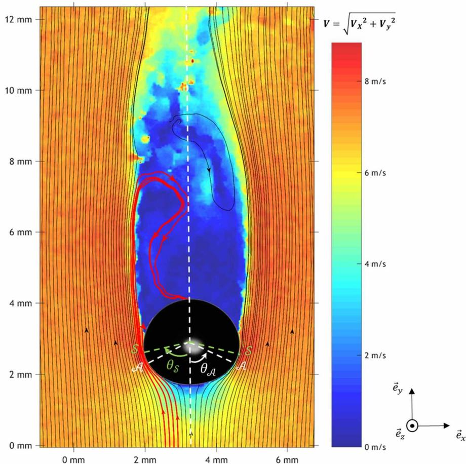
**Figure 8.** Instantaneous flow field around the drop measured using particle image velocimetry (PIV).  $V_x$  is the velocity component following  $\vec{e}_x$ , and  $V_y$  is the velocity component following  $\vec{e}_y$ .
