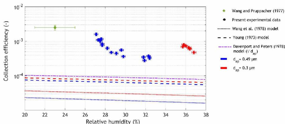
**Figure 6.** Comparison of measurements performed for this article with the various theoretical models in the literature for assessing the elementary contribution of phoretic effects—please note that in this figure, the Davenport and Peters model (1978) is independent of aerosol particle size. These simulations were performed assuming that the drop is in thermodynamic equilibrium with its environment. The drop interface temperature was determined using an enthalpy balance [4].
