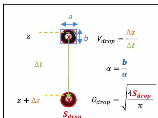
**Figure 2.** Measurement of the sizes, velocities, and axis ratios of drops.  $\Delta t$  is the time between two flashes,  $\Delta z$  is the distance crossed by the drop during  $\Delta t$ ,  $S_{drop}$  is the section of the drop,  $a$  and  $b$  are, respectively, the horizontal and vertical diameter of the drop.
