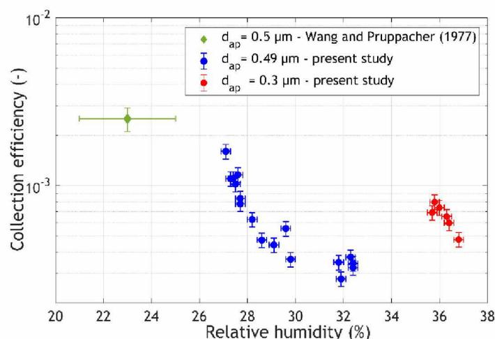
**Figure 5.** Measurement of the influence of relative humidity in the aerosol chamber on the collection efficiency of drops.
