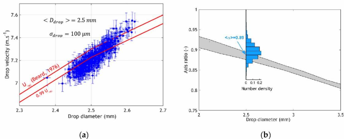
**Figure 3.** (a): correlation between drop size and velocity, and comparison with the theoretical terminal velocity established by Beard [52]. (b): Comparison of the distribution of axis ratios (bar graph in blue) measured in the aerosol chamber with mean axis ratios reported by Andsager (in grey) [55]. This area includes the mean axis ratios measured by Pruppacher and Beard [56] and the models of Pruppacher and Pitters [57], Green [58], and Beard and Chuang [59].
