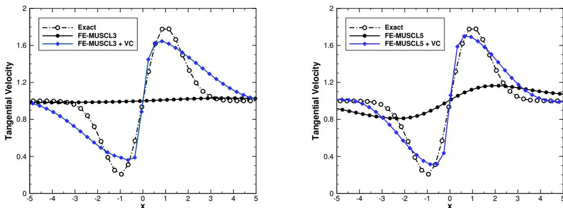
Figure 2. Comparison of tangential velocity profiles, centered at  $x = 0$ , for FE-MUSCL schemes with and without VC. Profiles after 30 passages across the domain for the 3<sup>rd</sup>-order schemes (left) and after 300 passages across the domain for the 5<sup>th</sup>-order schemes (right).
