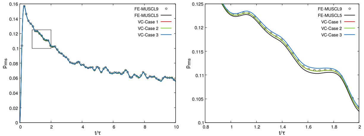
Figure 7. Comparison of the time evolution of r.m.s. pressure obtained with FE-MUSCL schemes with and without VC for initial turbulent Mach number  $M_{t0} = 0.5$ . Evolution during the complete computed time (left) and detail at  $t = 0.8\tau - 2\tau$  (right).
