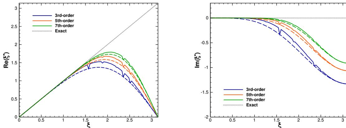
Figure 1. Spectral properties of FE-MUSCL schemes up to 7<sup>th</sup>-order of accuracy. Baseline schemes (dashed lines) and with confinement (solid lines),  $\varepsilon = 1.14 k_p$ . Taken from Ref.<sup>21</sup>
