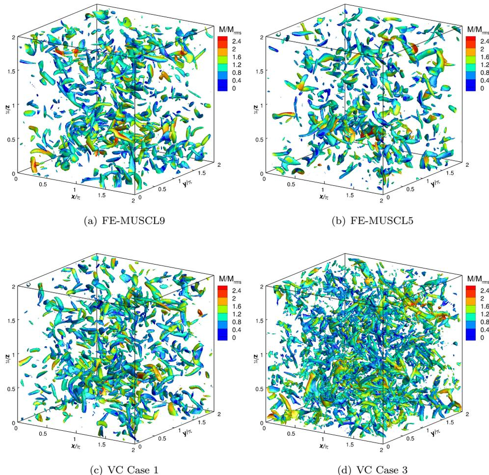
Figure 11. Iso-surfaces of constant vorticity magnitude at  $t = 10\tau$  colored by the local Mach number. Computed with FE-MUSCL schemes with and without VC on a  $128^3$  grid for initial turbulent Mach number  $M_{t0} = 0.2$ .
