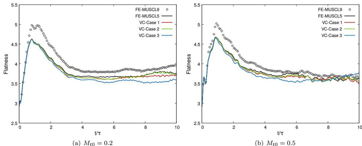
**Figure 9.** Comparison of the time evolution of the flatness factor of the fluctuating velocity gradient distribution obtained with FE-MUSCL schemes with and without VC for the two different initial turbulent Mach number cases.
