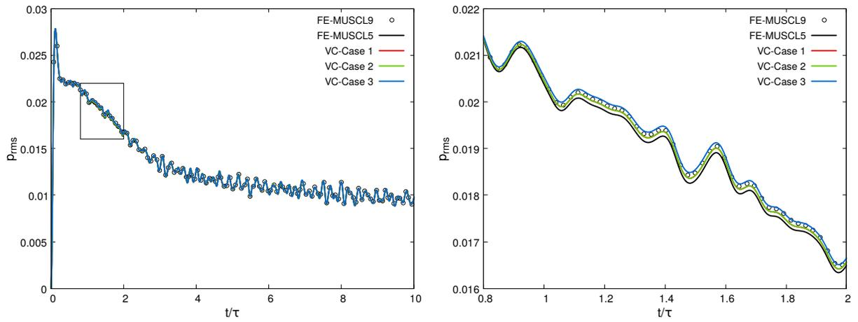
Figure 6. Comparison of the time evolution of r.m.s. pressure obtained with FE-MUSCL schemes with and without VC for initial turbulent Mach number  $M_{t0} = 0.2$ . Evolution during the complete computed time (left) and detail at  $t = 0.8\tau - 2\tau$  (right).
