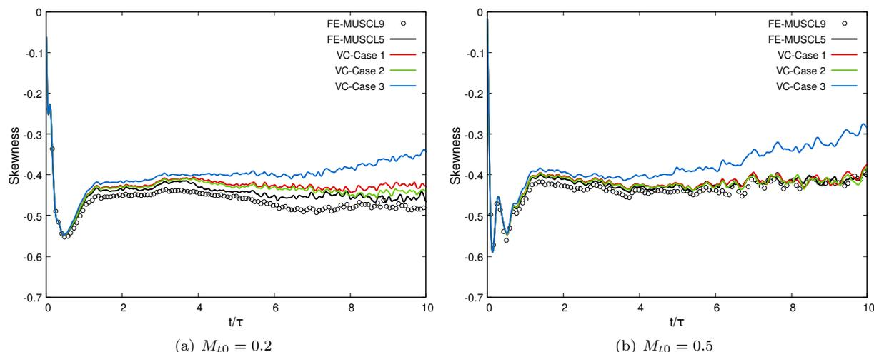
**Figure 8.** Comparison of the time evolution of the skewness factor of the fluctuating velocity gradient distribution obtained with FE-MUSCL schemes with and without VC for the two different initial turbulent Mach number cases.
