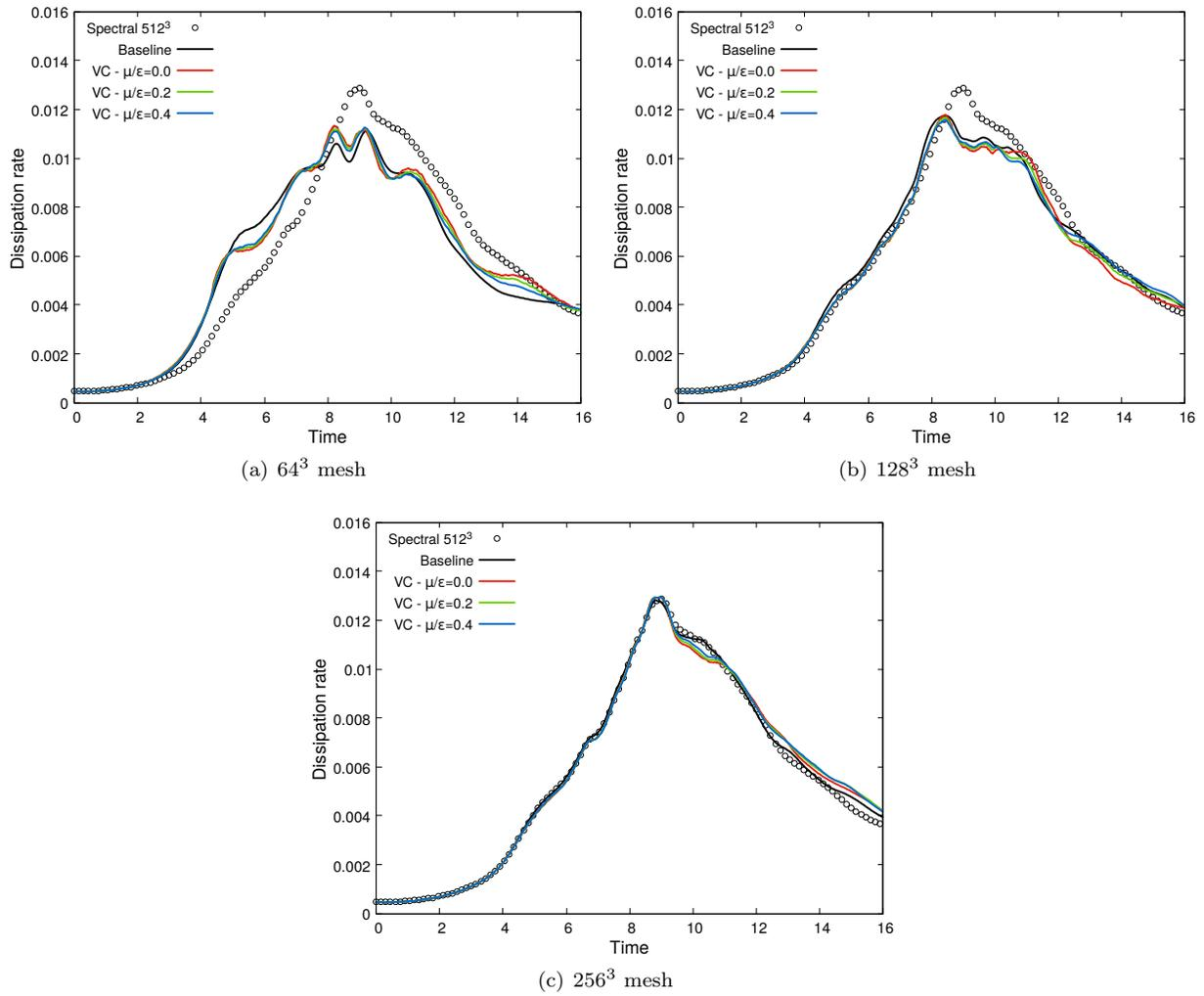
Figure 3. Effect of VC on the evolution of the kinetic energy dissipation rate for the Taylor-Green vortex case and sensitivity to the value of  $\mu/\epsilon$ . FE-MUSCL5 and 5<sup>th</sup>-order Vorticity Confinement.
