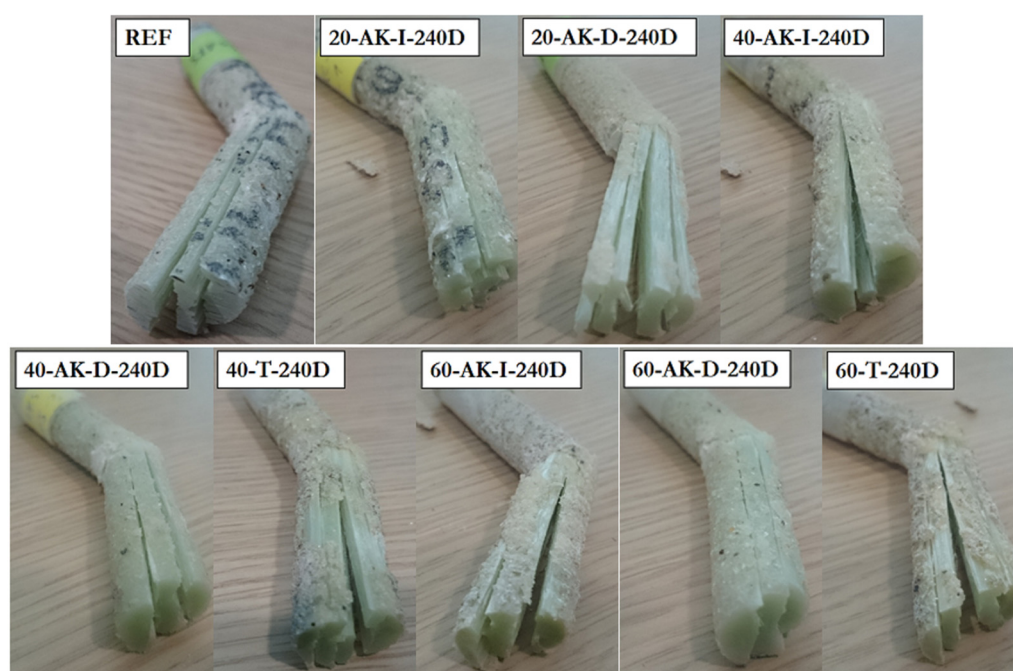
Figure 16. Failure modes observed after short-beam tests on reference and aged GFRP rebars.
