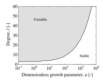
Figure 6: Degree, l, of the spherical harmonic function,  $Y_{(l)}^{(m)}$ , associated to the development of instabilities with the relative stability criterion as a function of the dimensionless growth parameter.
