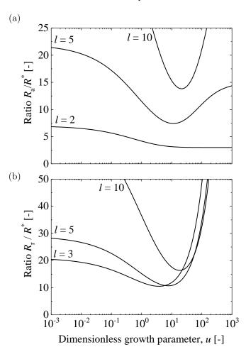
Figure 3: Evolution of the threshold radius defining the growth stability of a spherical particle considering both (a) the absolute stability criterion,  $R_a$ , and (b) the relative stability criterion,  $R_r$ , as a function of the dimensionless growth parameter u for a binary alloy. Curves are normalized by the critical nucleation radius,  $R^*$ , and are drawn for several values of the degree of the spherical harmonics, l.
