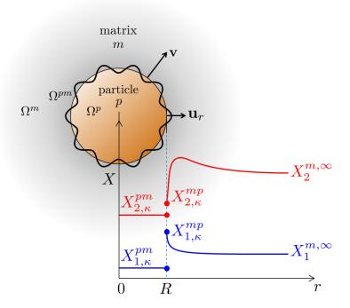
Figure 1: Illustration of (orange) a particle phase, p, embedded in (grey) a matrix phase, m, at a given temperature, T, together with schematized molar composition profiles for (blue) component 1 and (red) component 2 in both domains  $\Omega^p$  and  $\Omega^m$ . The interface separating the two domains,  $\Omega^{pm}$ , is schematized by a black line for both (thin) a stable spherical particle shape and (thick) a perturbed form at the onset of instability.
