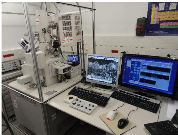
Figure 9: Analysis of samples by SEM-EDS in progress.
