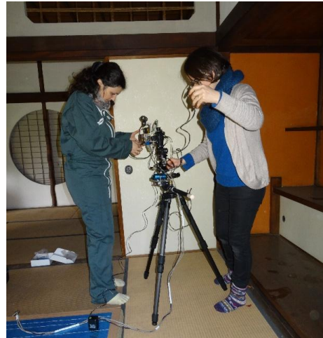
Figure 7: Preparation of the fluorescence X machine for in situ measurements. (Photo : C. Lavier)
