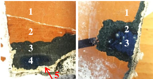
Figure 2: Left: we have scoured only 5 of the 10 layers; Right: only 3 from 8 present layers.
