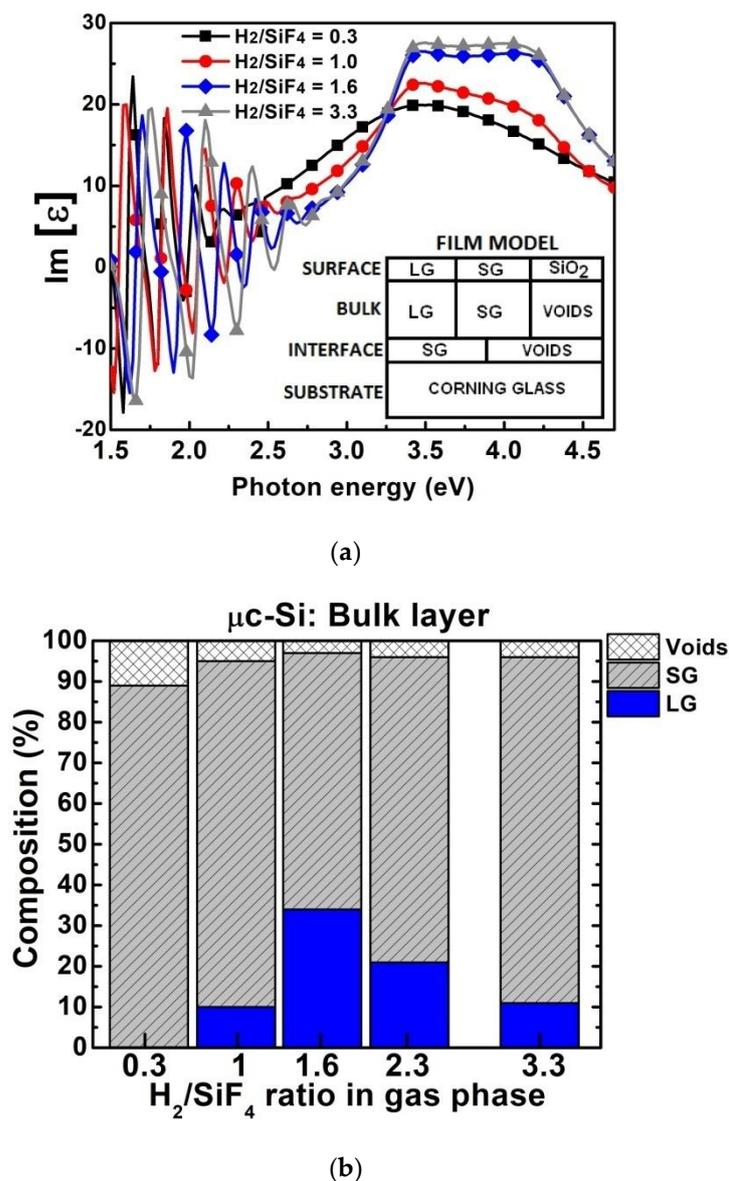
**Figure 2.** (a) Imaginary part of the pseudo-dielectric function ( $\text{Im}[\epsilon]$ ) of  $\mu\text{c-Si:H,F}$  films deposited with a  $\text{H}_2/\text{SiF}_4$  gas ratio 0.3–3.3 on corning glass substrates. The inset shows the  $\mu\text{c-Si:H,F}$  film optical model. (b) Composition of  $\mu\text{c-Si:H,F}$  bulk films deposited on corning glass as a function of the  $\text{H}_2/\text{SiF}_4$  gas ratio (obtained from modeling the  $\text{Im}[\epsilon]$  spectra).
