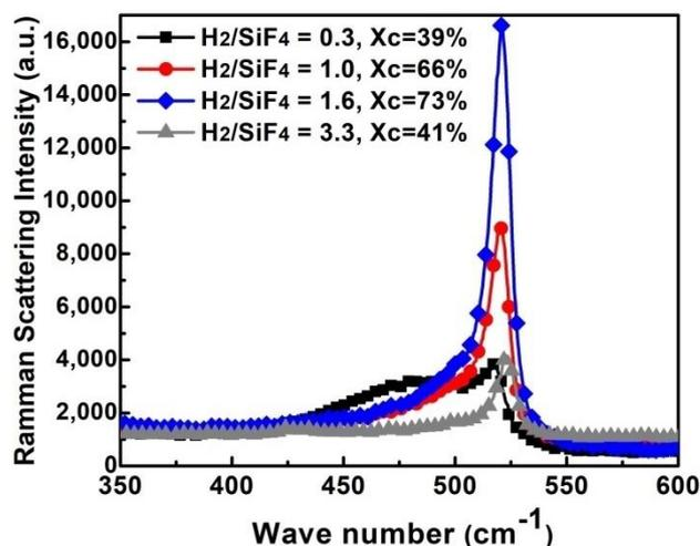
Figure 1. Raman spectra of  $\mu\text{c-Si:H,F}$  films deposited with a H<sub>2</sub>/SiF<sub>4</sub> gas ratio of 0.3–3.3.
