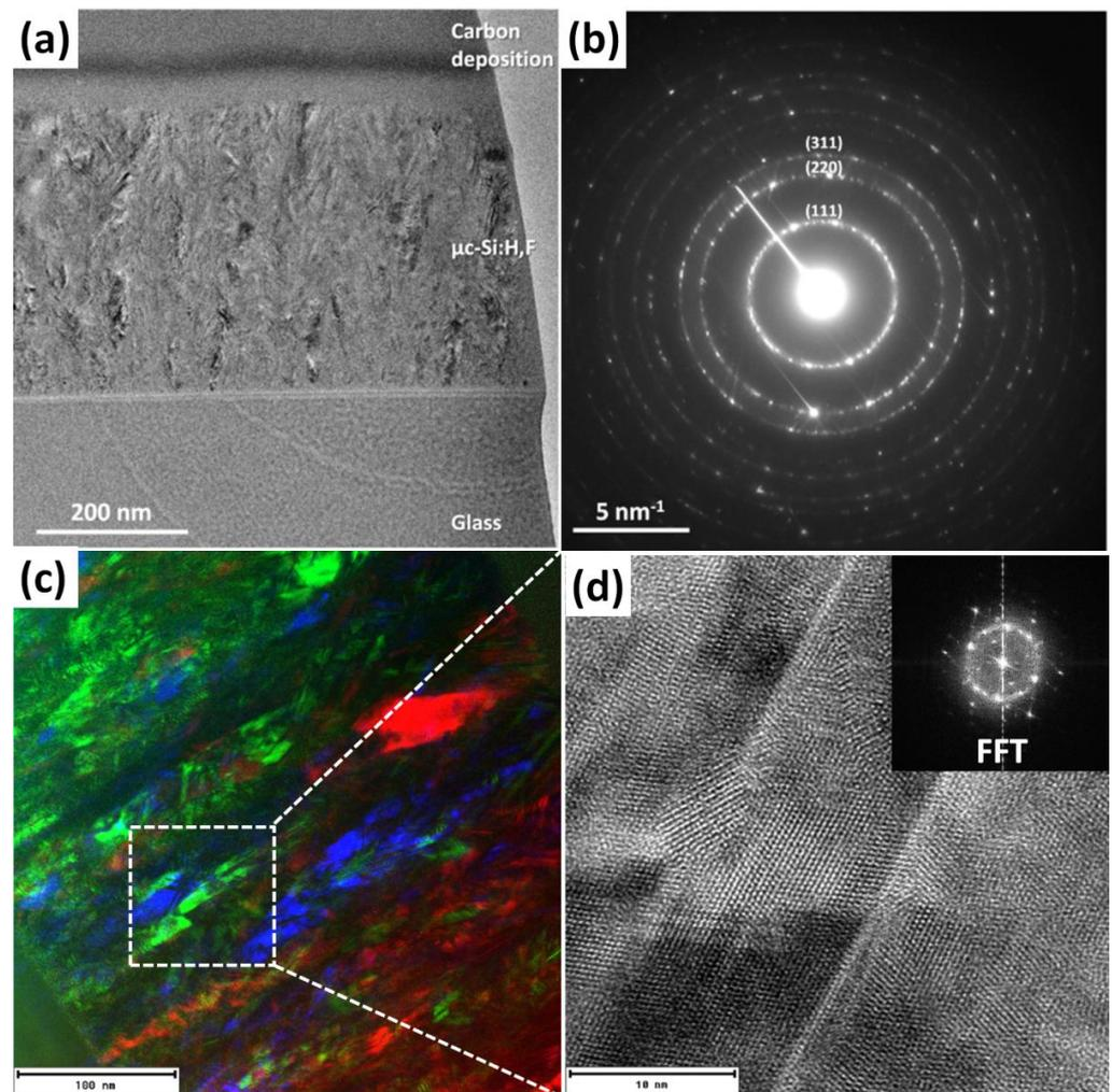
**Figure 3.** (a) TEM image of the  $\mu\text{c-Si:H,F}$  film, with the largest LG fraction (34%), and (b) SAED pattern of the film showing the characteristic planes of the Si structure. (c) RGB image formed by three dark field juxtaposed images collected with different positions of the objective lens aperture, and (d) HRTEM image of the selected area and their corresponding FFTs revealing the crystalline structure.
