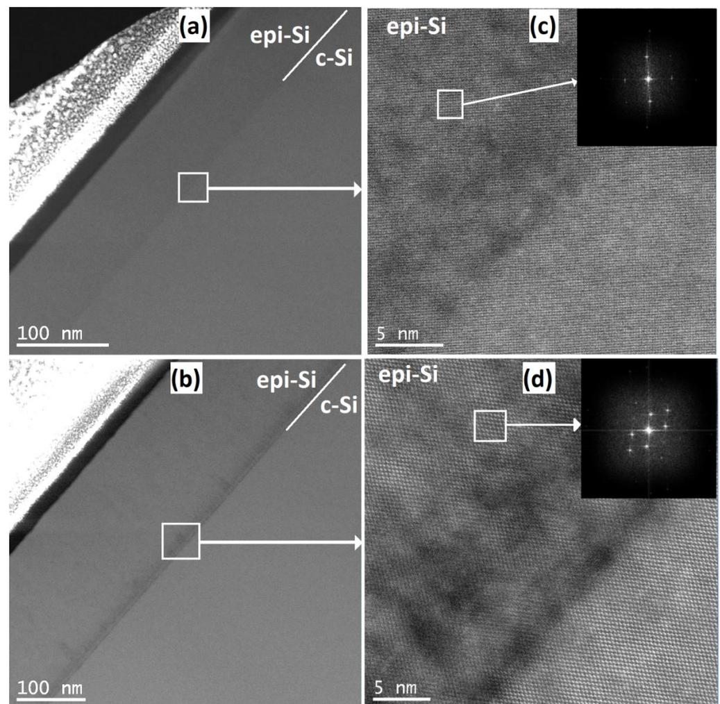
**Figure 6.** STEM cross sectional view of the epi-Si/silicon interface for the  $H_2/SiF_4$  ratios of (a) 0.3 and (b) 1. HRSTEM on the black square region for the epi-Si films deposited using  $H_2/SiF_4$  with mixing ratios of (c) 0.3 and (d) 1.
