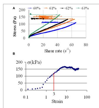
**FIGURE 2 | (A)** Rheogram of carbonyl iron suspensions with 0.2% of superplasticizer at high-volume fraction (blue:60%, orange 61%, black 62%, green 63%). **(B)** Stress vs. strain in cylindrical Couette geometry with vane tool,  $\Phi = 0.61$ ;  $H_0 = 19.2$  kA/m, The vertical red line corresponds to a time of 2 s where the shear rate has reached its final value of 1.6 s  $^{-1}$ .
