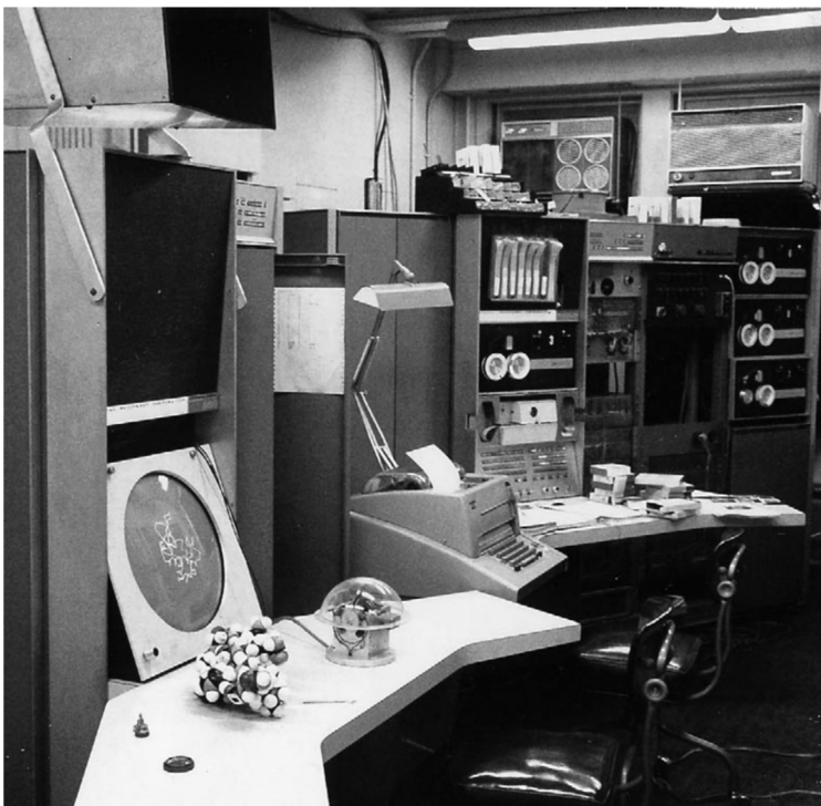
Figure 3. The setup of Levinthal's pioneering machine with the DEC 340 graphics console and a "globe" that controls the direction and speed of image rotation in the foreground. In the back is the PDP-7 minicomputer, and in the centre is the standard remote control console. Reproduced with permission from , image courtesy of Martin Zwick.
