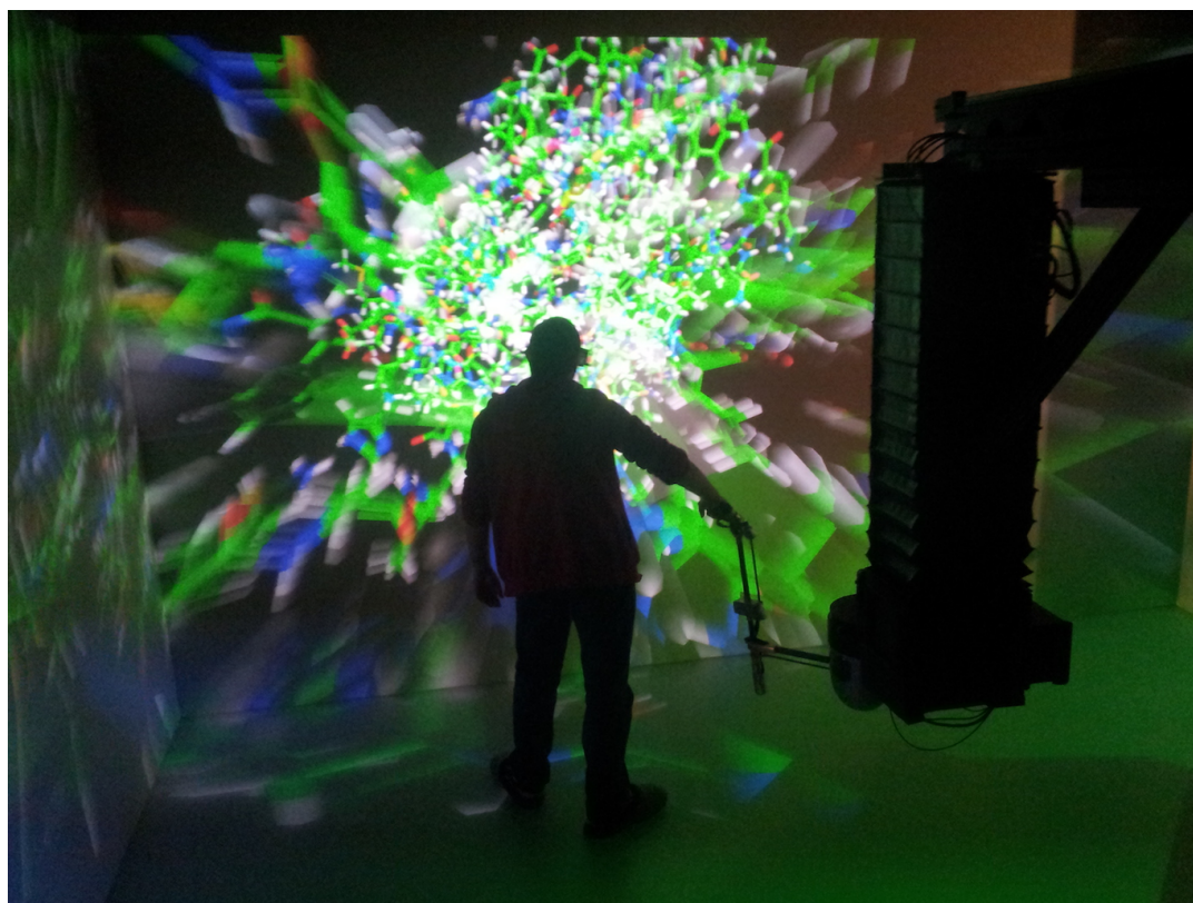
Figure 8. User performing an interactive molecular simulation in a CAVE environment that has an advanced haptic device with access to the entire workspace of the immersive system.
