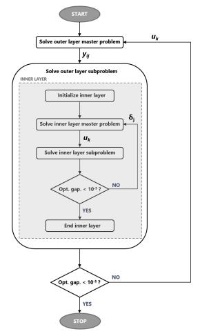
Fig. 1: Flowchart of the NC&CG algorithm.
