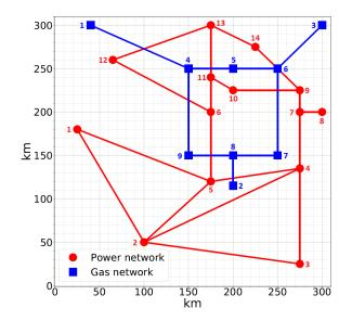
Fig. 2: Geographical allocation of the interdependent power and gas network.
