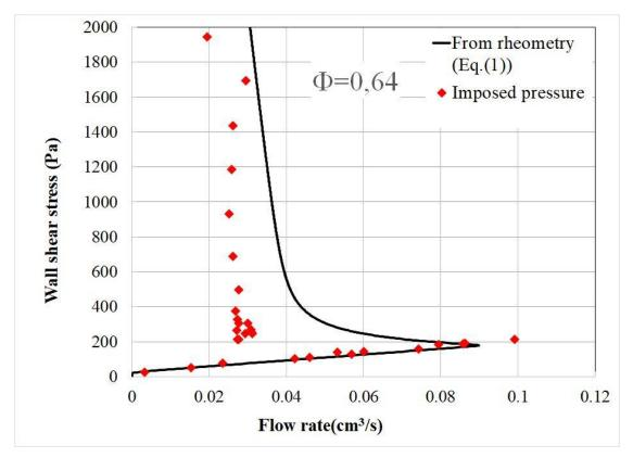
**Fig.4** Volume fraction  $\Phi$ =0.64. Red dots are the flow rates measured at different imposed pressures. The solid line is obtained from Eq. (1) with  $\dot{\gamma}(\tau)$  given by the dashed curve of Fig. (2) for  $\Phi$ =0.64.
