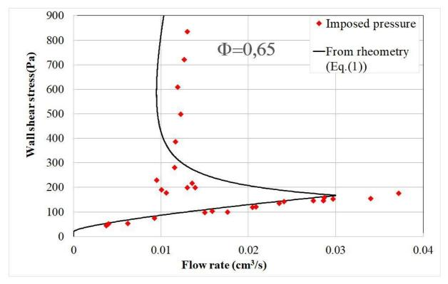
**Fig.5** Volume fraction  $\Phi$ =0.65. Red dots are the flow rates measured at different imposed pressures. The solid line is obtained from Eq. (1) with  $\dot{\gamma}(\tau)$  given by the dashed curve of Fig. (2) for  $\Phi$ =0.65.
