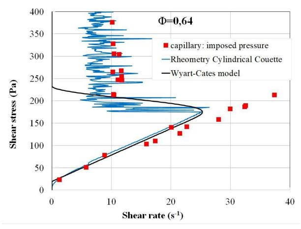
**Fig.6** Fit of the rheometric curve (blue solid line) by the Wyart-Cates model (solid black line). The shear rate for the results at imposed pressure (red squares) is deduced from the flow rate by: $\dot{\gamma} = 4Q/(\pi R^3)$
