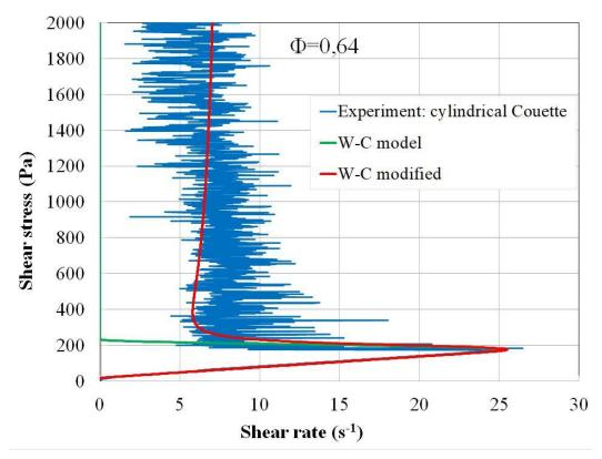
**Fig.8** Comparison of the prediction of the W-C model (green line) with the modified value of *f*: Eq. (6) and  $t_L=0.18s$  (red line). The solid blue line is the experimental result in Couette geometry at  $\Phi=0.64$ .
