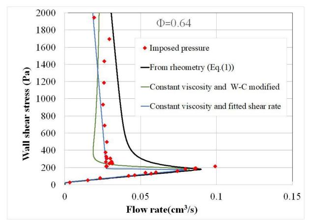
**Fig.9** Different models used to predict the volume flow rate at imposed pressure. Solid black line: Eq. (1) with fitted value of  $\dot{\gamma}(\tau_R)$  (cf. Fig. (2)). Green solid line: Eq. (7) with  $\dot{\gamma}(\tau_R)$  from the modified W-C model. Blue solid line: Eq. (7) with the fitted values of  $\dot{\gamma}(\tau_R)$ . Red dots: experimental points at  $\Phi$ =0.64.
