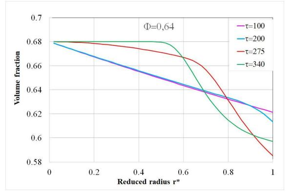
Fig. (10)) Predicted volume fraction profiles  $\Phi(r^*)$  for four different wall stresses:  $\tau$ =100Pa,  $\tau$ =200Pa,  $\tau$ =275Pa,  $\tau$ =340Pa at an average volume fraction of  $\Phi$ =0.64
