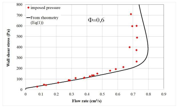
**Fig.3** Volume fraction  $\Phi$ =0.6. Red dots are the flow rates measured at different imposed pressures. The solid line is obtained from Eq. (1) with  $\dot{\gamma}(\tau)$  given by the dashed curve of Fig. (2) for  $\Phi$ =0.6.
