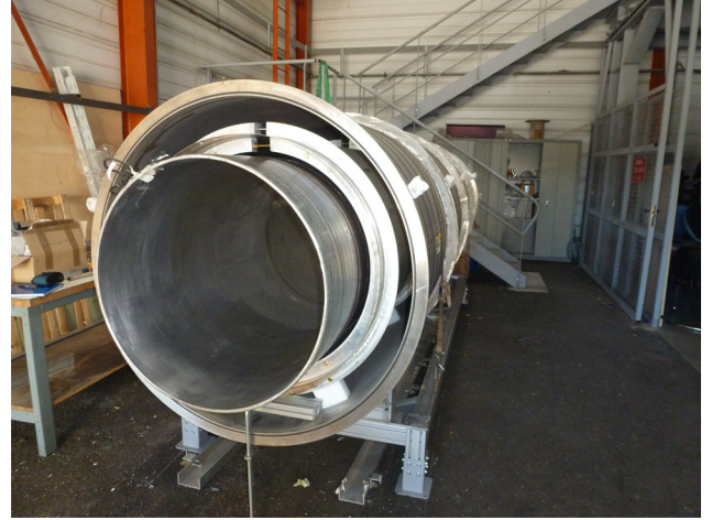
FIG. 1 (color online). Solenoid inserted into the mumetal magnetic shield.
