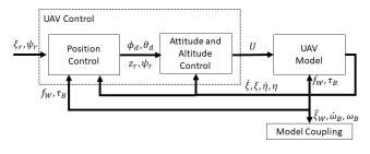
Fig. 3. UAV hierarchical control.
