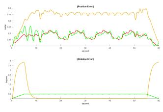
Fig. 8. End effector trajectory error with disturbance on UAV.
