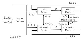
Fig. 2. Full block diagram of a coupled system.
