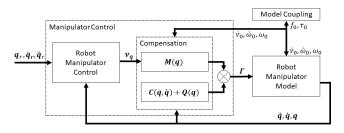
Fig. 4. Manipulator computed torque control.
