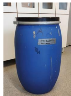
Fig. 2. The barrel used in a project. The size of the barrel was determined to achieve the optimal stirring. The homogeneous sediment masses were obtained for further testing. Photo by Per Lindh
