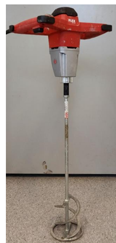
Fig. 3. Mixing tool for the homogenisation of the dredged material. Photo by Per Lindh
