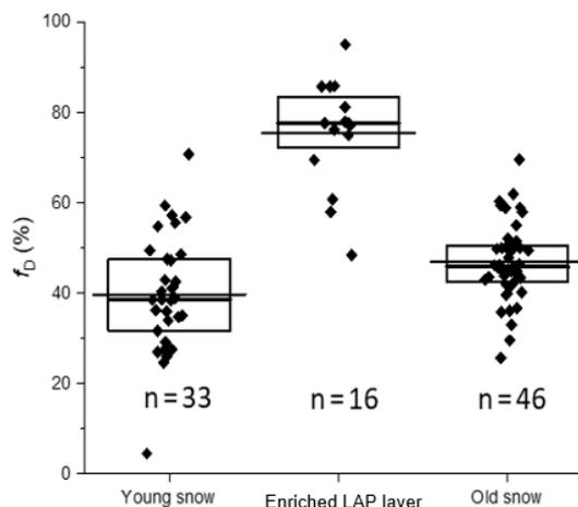
**Figure 5.** Fractional dust absorption remaining after burning the filters during OCEC analysis. The diamonds are individual values for each filter, and the thin extended line represents the arithmetic average. The box and thicker line represent the quartile range and median, respectively. The number of samples is indicated in the figure as  $n$ .
