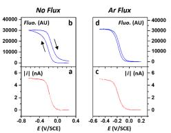
**Figure 1.** Cyclic voltammetry and voltfluorometry of the HPTS/BQ fluorogenic system. (a, c) Cyclic voltammogram (CV) of 1 mM BQ in the presence of 2 mM HPTS, at a 25  $\mu$ m diameter carbon UME. (b, d) Simultaneously recorded voltfluorograms (CVF). Effect of convection induced by an argon flux blown over the solution: (a, b) flux off, (c, d) flux on. 0.1 M KCl aqueous electrolyte, scan rate 0.01 V s<sup>-1</sup>.
