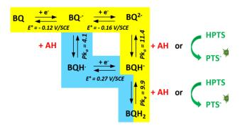
Scheme 3. Square scheme depicting the possible reduction paths for benzoquinone (BQ) at an electrode, in the presence of an acid (AH) and HPTS.
