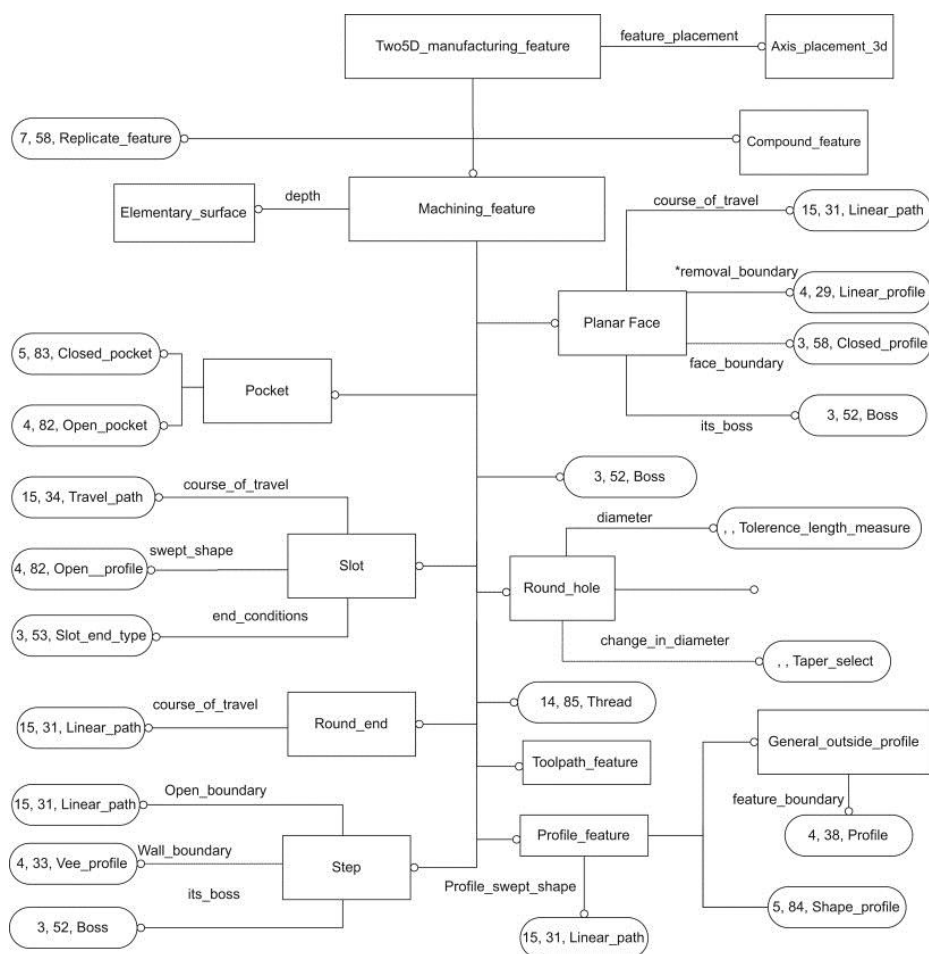
Figure 1: EXPRESS-G representation of manufacturing feature in STEP-NC [6]
