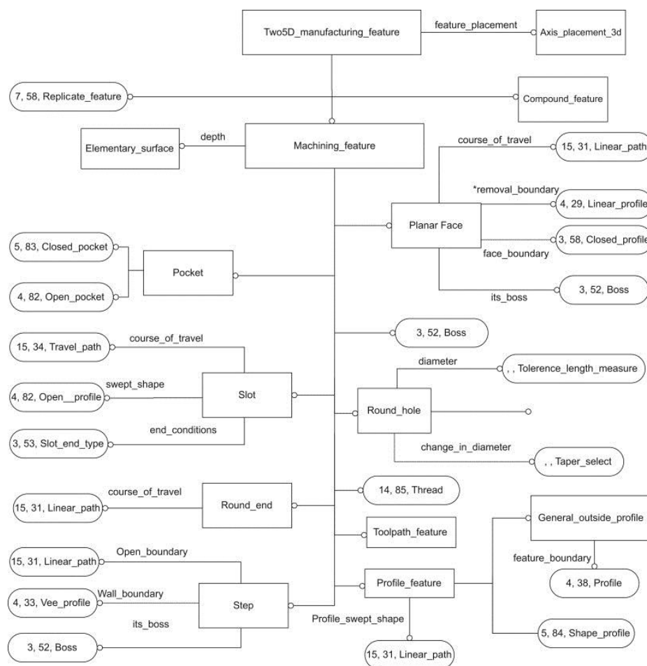
Figure 1: EXPRESS-G representation of manufacturing feature in STEP-NC [6]
