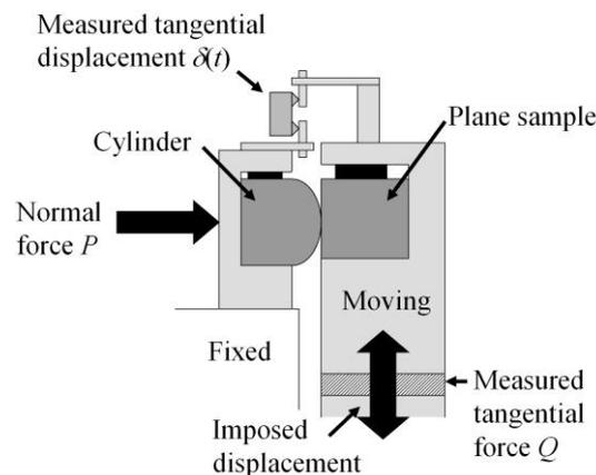
**Figure 2-** Basic sketch of a plain fretting test.
