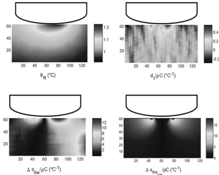
Figure 6- First estimation of the heat sources.
