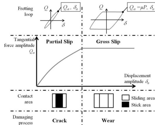
**Figure 1-** Basic sketch of plain fretting sliding conditions.
