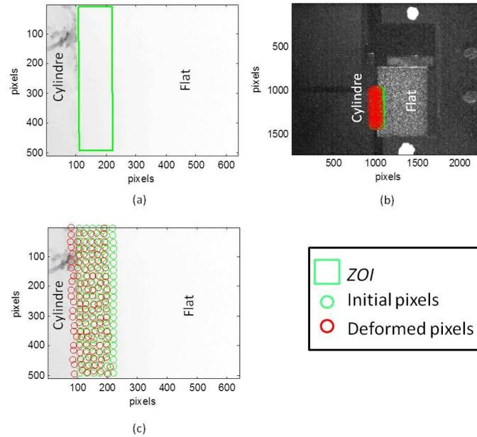
**Figure 4-** Images processing: (a) ZOI selection on IR image, (b) In-plane displacements determination using DIC technique, (c) new deformed ZOI.
