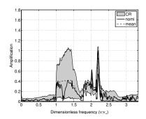
**Figure 1:** Stochastic analysis: frequency domain observation  $Y^{\text{NL}}(2\pi\nu)$  related to the nonlinear case for a moderate mistuning rate mean model (thick line), confidence region (gray region).
