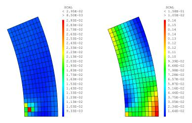
Figure 7 – Error estimated by the ZZ estimator (at left) and error between the finite element solution and the reference solution (at right) (mesh size :  $109 \mu m$ )
