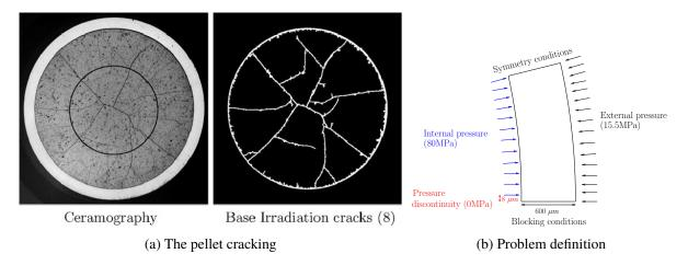
FIGURE 5 – 2D (r, $\theta$ ) test case
