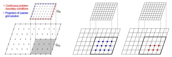
Figure 3 – Example of boundary conditions on  $G_h$  for hierarchical meshes
