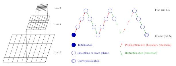
FIGURE 1 – Example of hierarchical meshes used in LDC method
