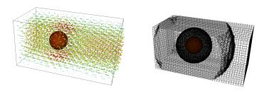
Figure 4: Flow around the ball and AMR mesh
