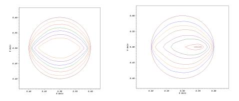
Figure 8: Erosion of soil cylinder for Stokes and Navier-Stokes flows
